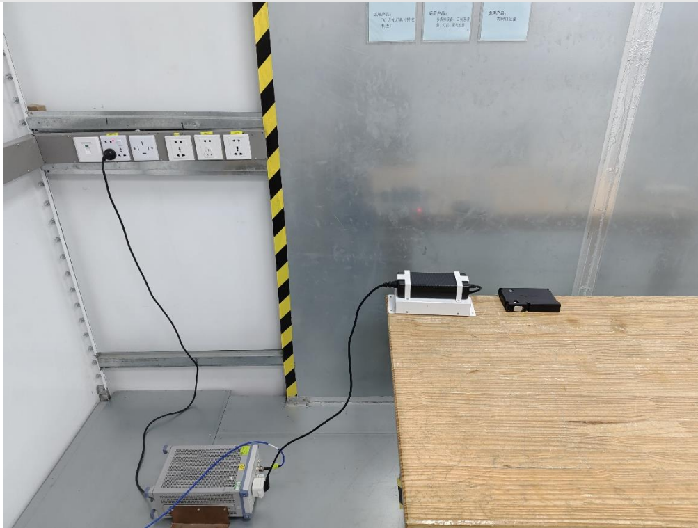
AC Power Line Conducted Emission
