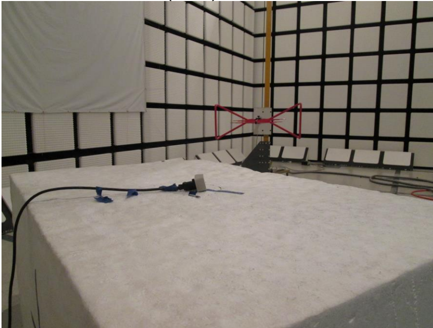
RADIATED EMISSIONS (BACK)
