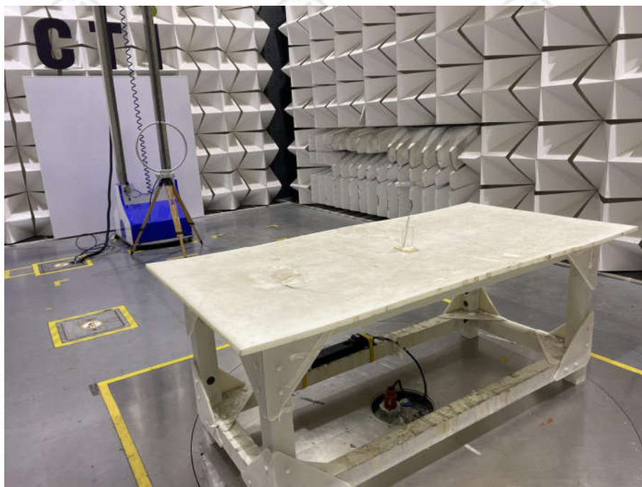
Radiated spurious emission Test Setup-1(Below 30M)
