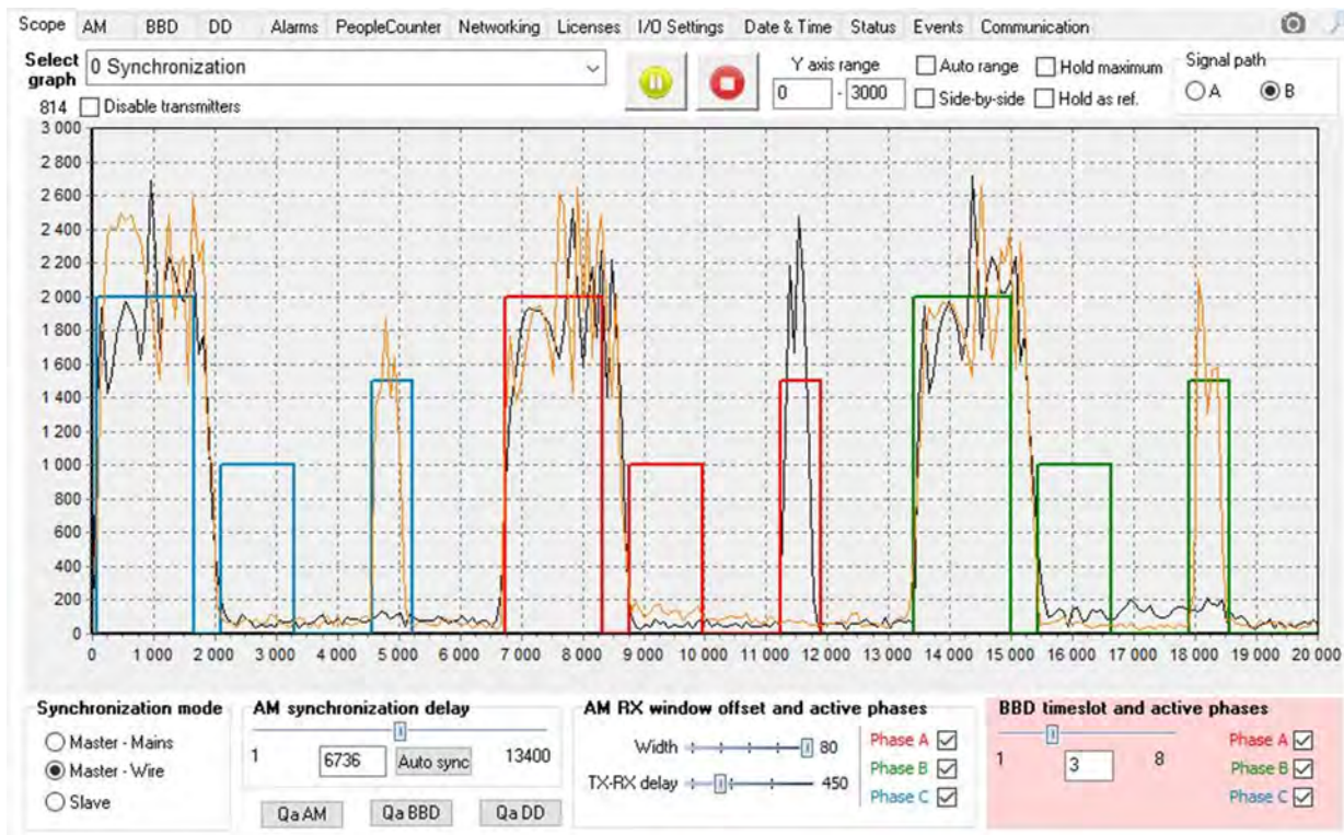
Picture 37 - Correctly synchronized system with booster bag
