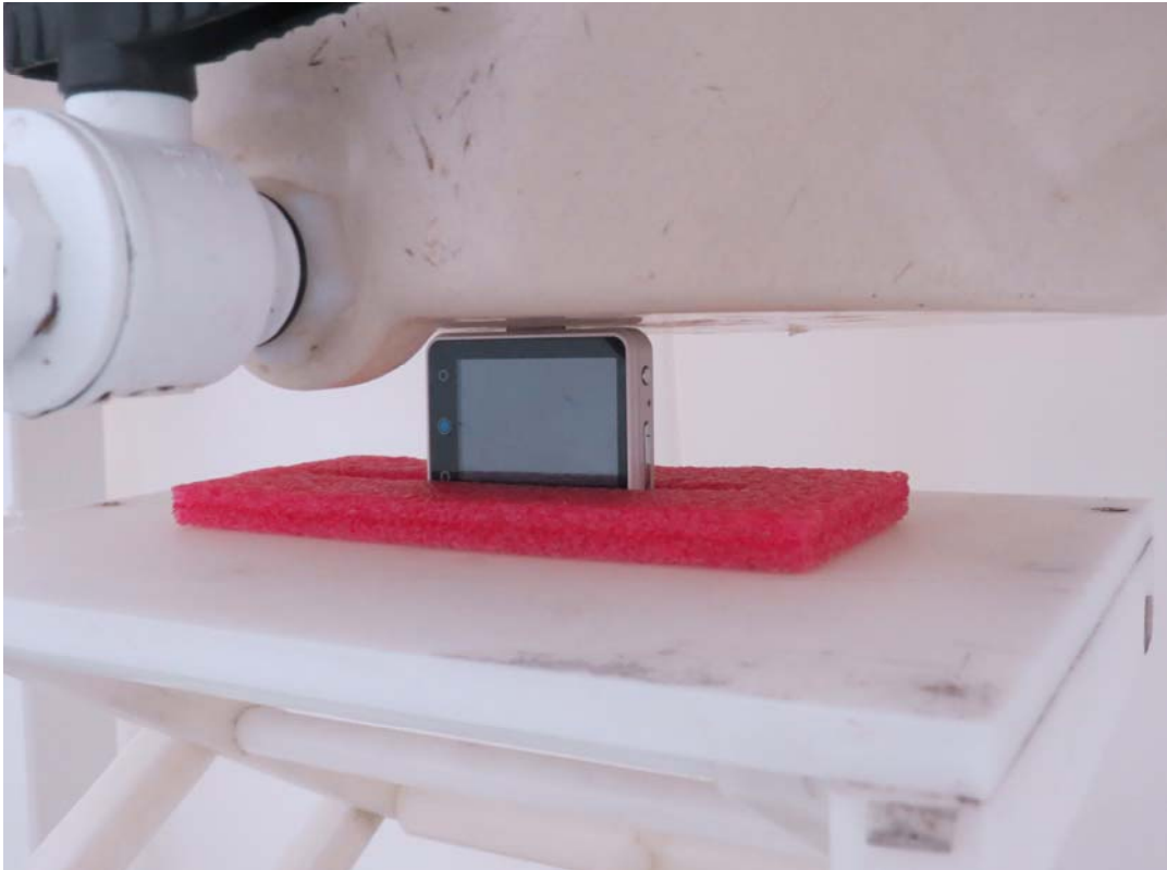
Picture 17: Bottom Edge without strap attached, the distance from handset to the bottom of the Phantom is 0mm
