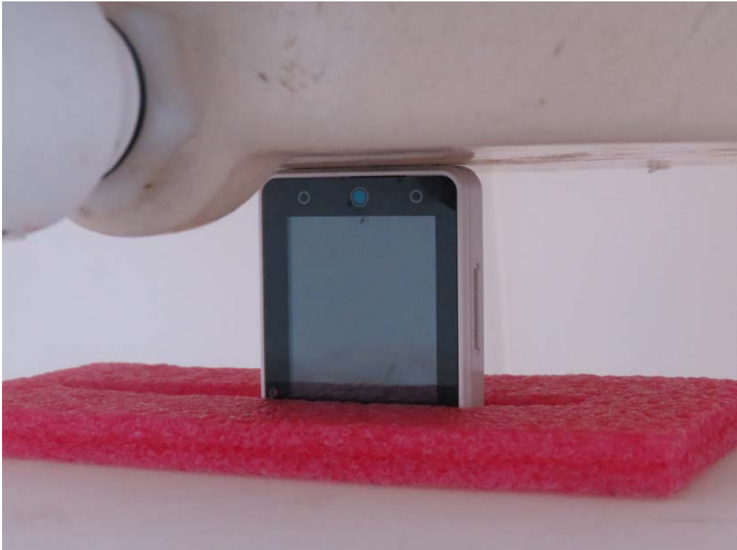
Picture 15: Right Edge without strap attached, the distance from handset to the bottom of the Phantom is 0mm
