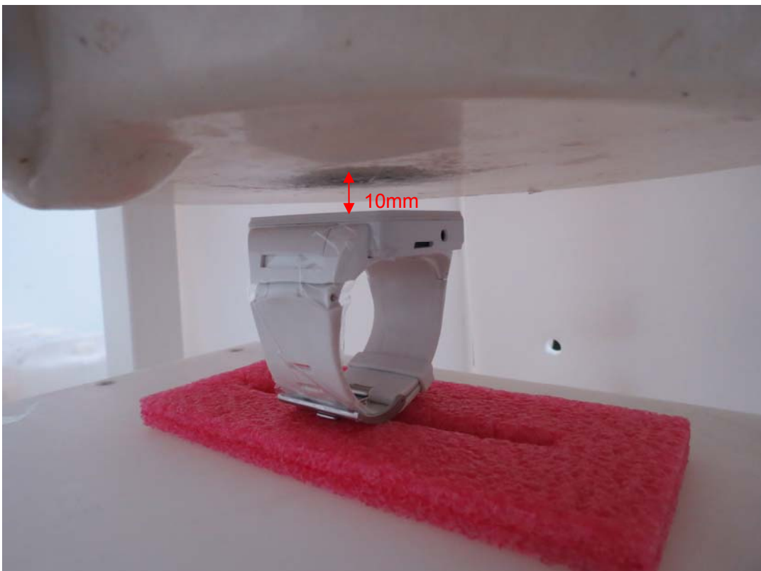
Picture 14: Front Side with strap attached, the distance from handset to the bottom of the Phantom is 10mm
