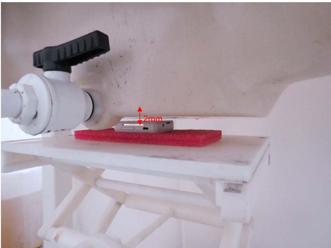
Picture 12: Back Side without strap attached, the distance from handset to the bottom of the Phantom is 2mm
