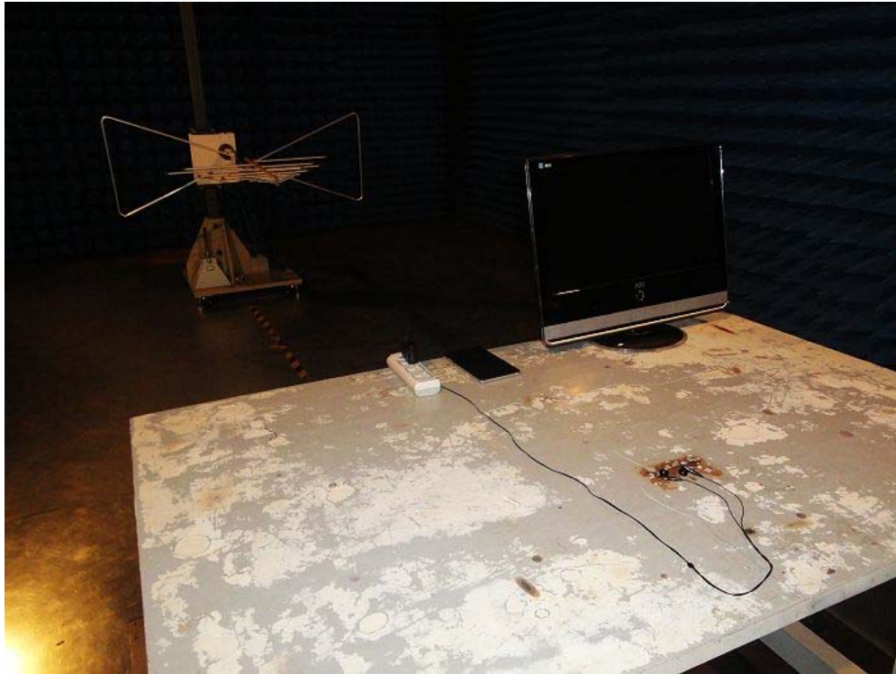
Radiated Emission Test Setup:
