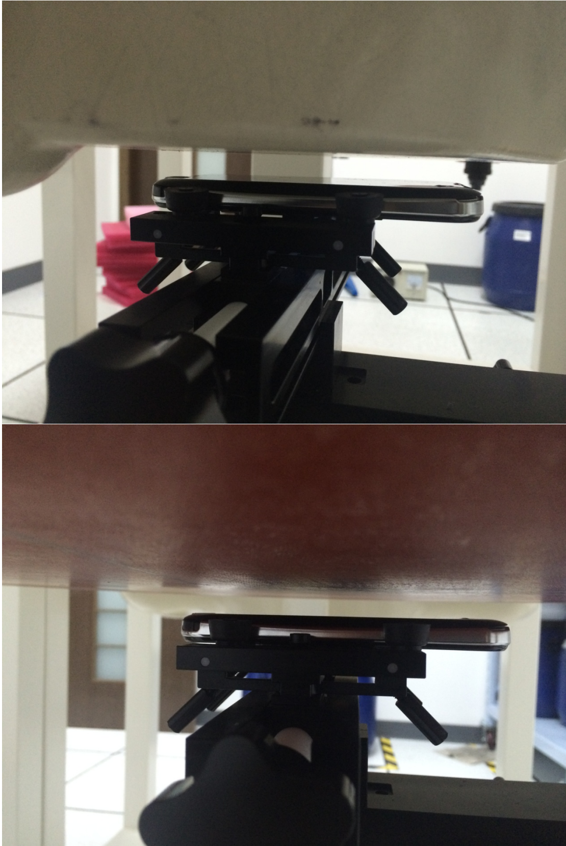
Band850, Band1900, WCDMA Band II and WIFI Test Setup Body Back with gap 10mm
