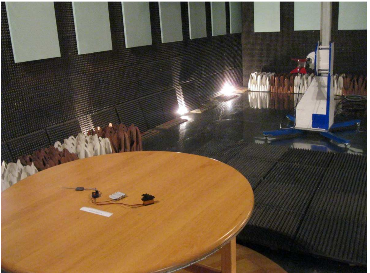
Figure 2.6.3 - Radiated Emission Test (Frequency Range 1 GHz – 18 GHz)
