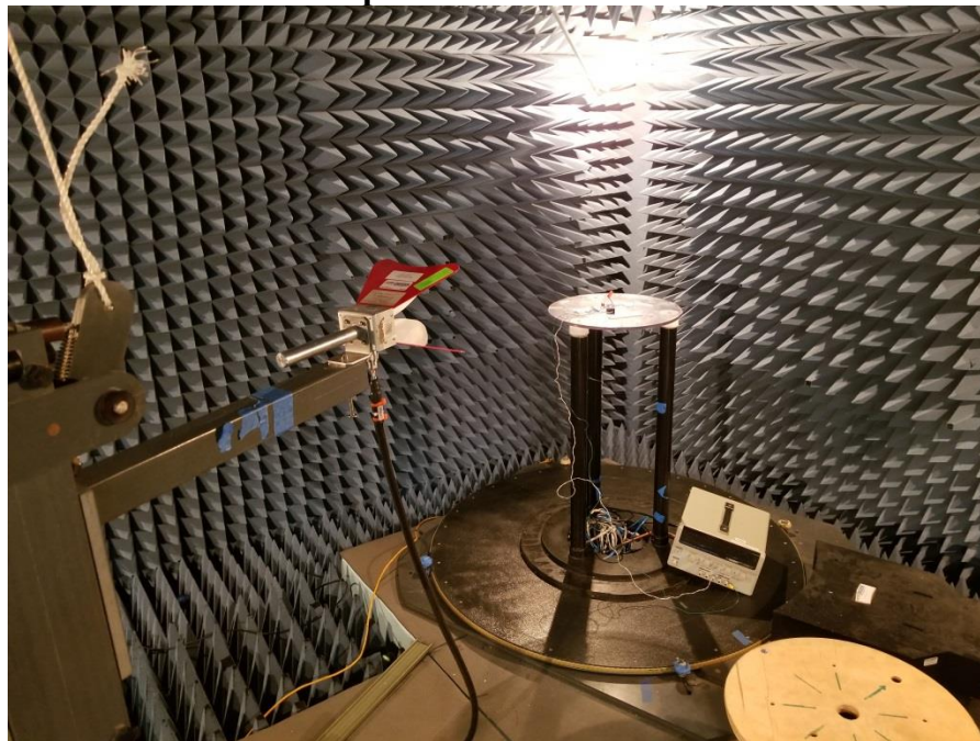
Photograph 1. Radiated Spurious Emissions, Above 1 GHz, Test Setup
