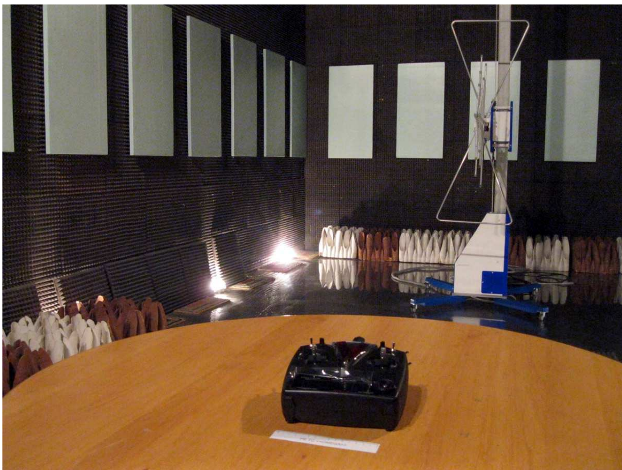
Figure 2.6.2 - Radiated Emission Test (Frequency Range 30 MHz – 1000 MHz)
