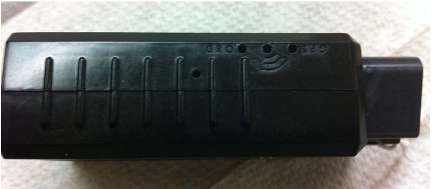
Side 4 of 6 (Three holes are for LED status indicators.)
