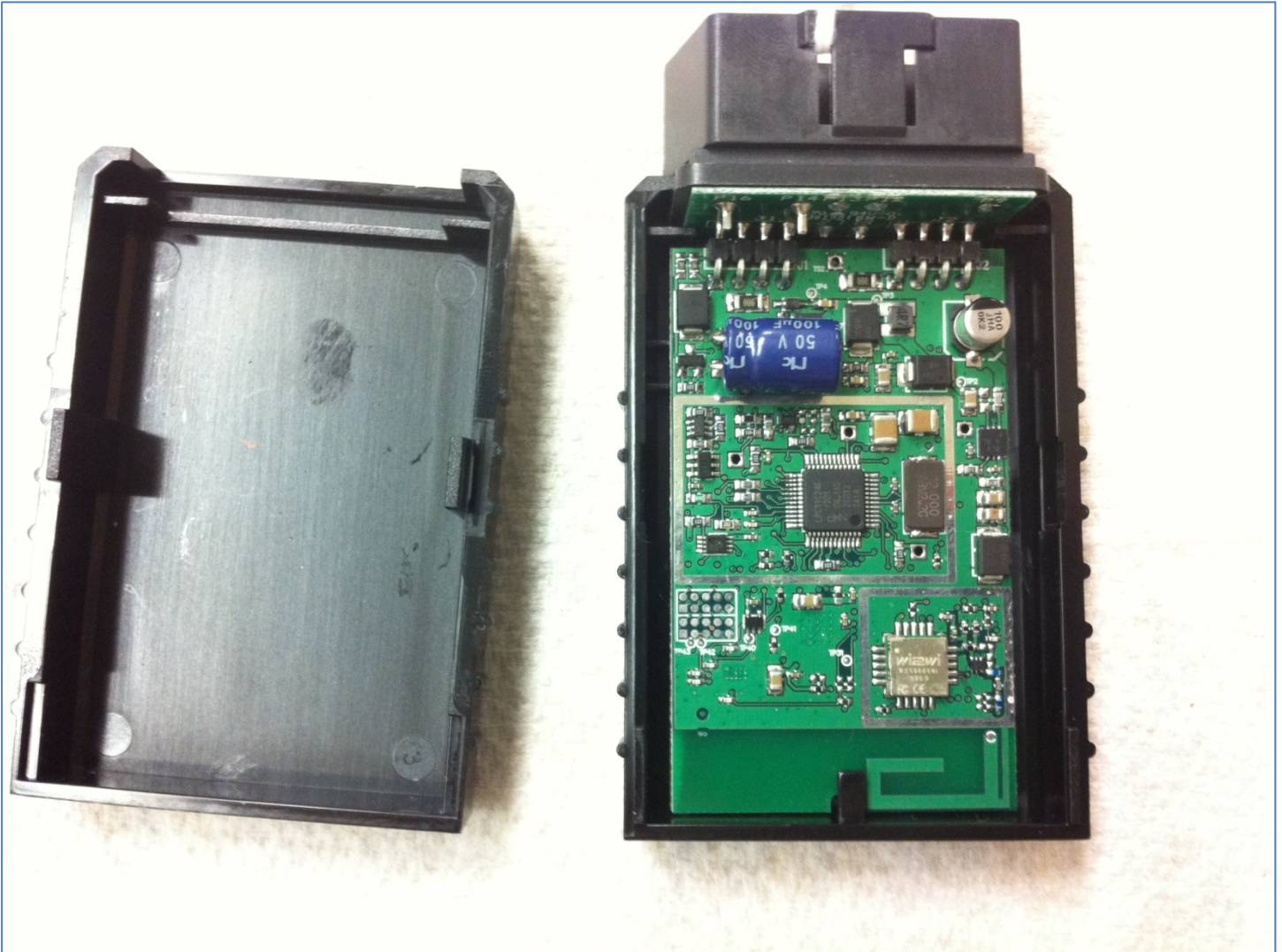
Enclosure Open Revealing Location of Circuit Boards
