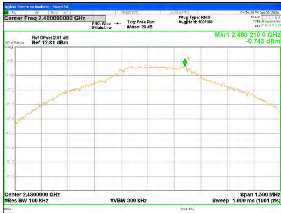
Tx. Spurious NVNT 1-DH5 2480MHz Ant1 Ref
