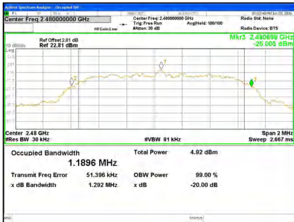
-20dB Bandwidth NVNT 2-DH5 2480MHz Ant1
