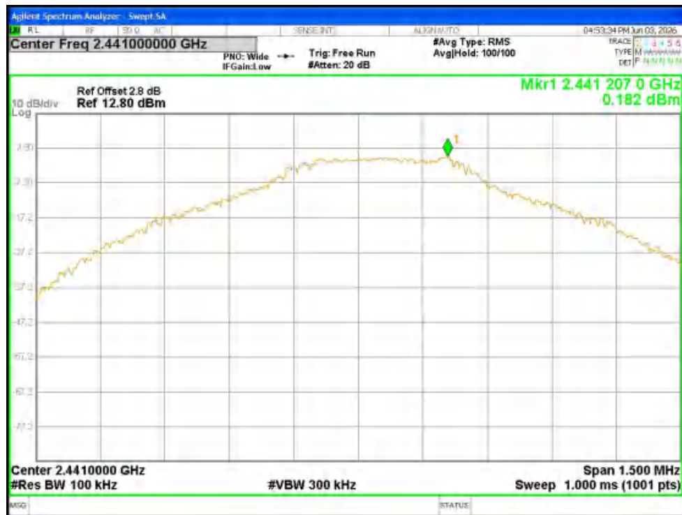
Tx. Spurious NVNT 1-DH5 2441MHz Ant1 Ref
