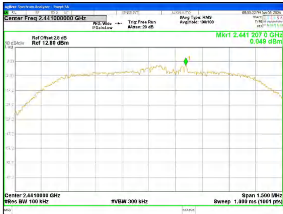
Tx. Spurious NVNT 2-DH5 2441MHz Ant1 Ref
