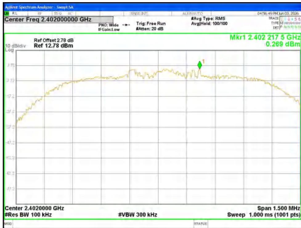
Tx. Spurious NVNT 2-DH5 2402MHz Ant1 Ref
