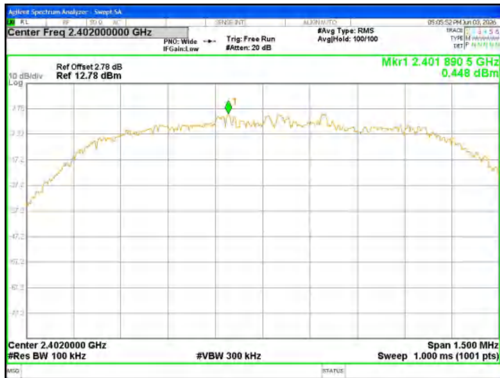
Tx. Spurious NVNT 3-DH5 2402MHz Ant1 Ref
