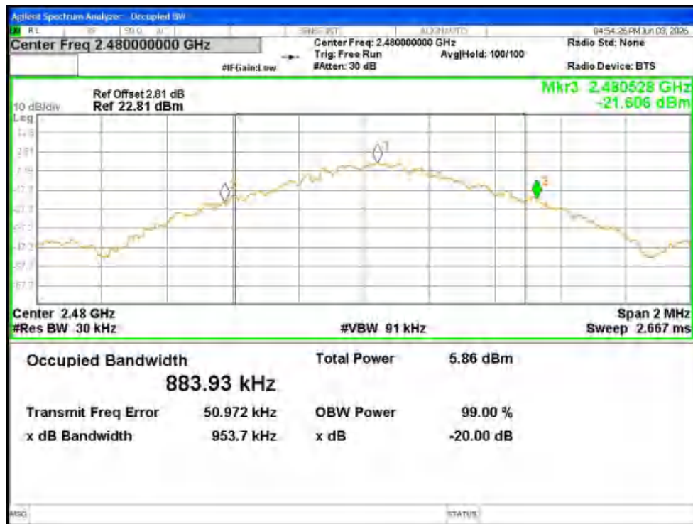
-20dB Bandwidth NVNT 1-DH5 2480MHz Ant1
