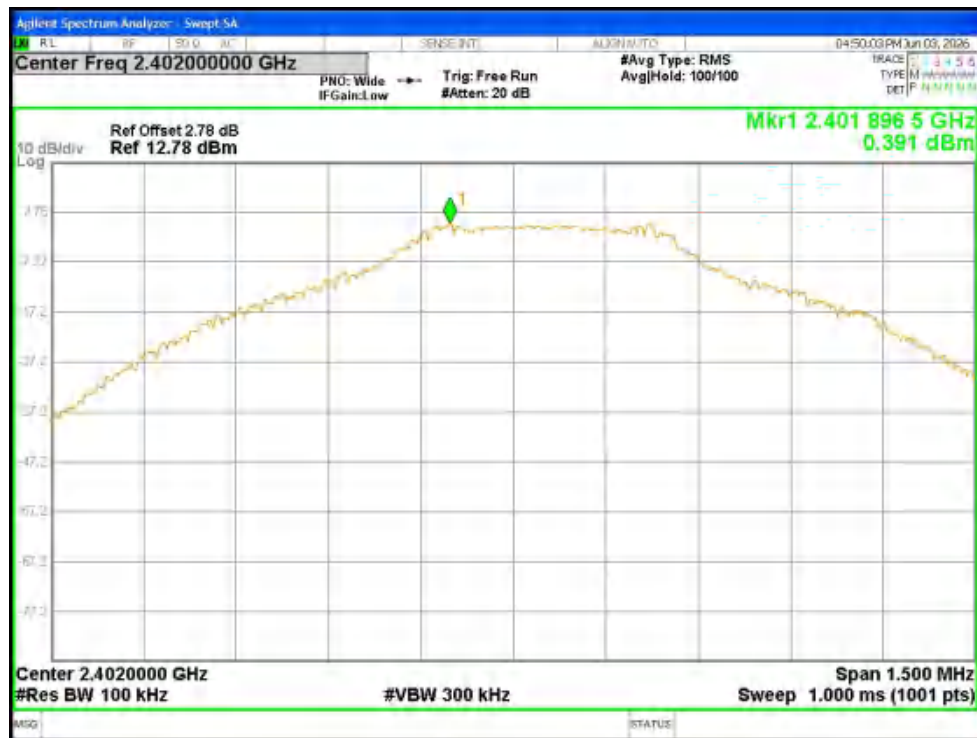
Tx. Spurious NVNT 1-DH5 2402MHz Ant1 Ref
