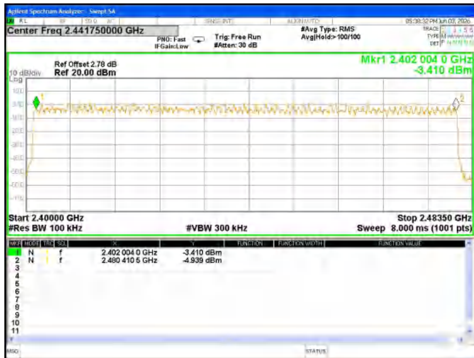
Hopping No. NVNT 3-DH5 2402MHz Ant1
