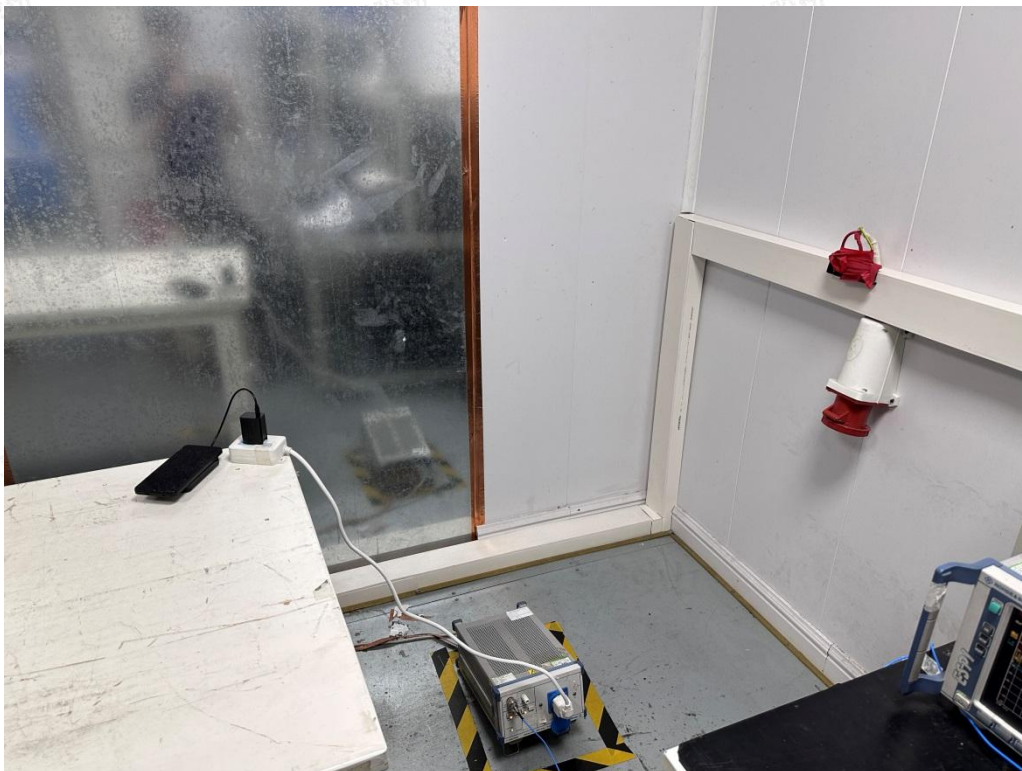
Conducted Emission-AC adapter charge mode
