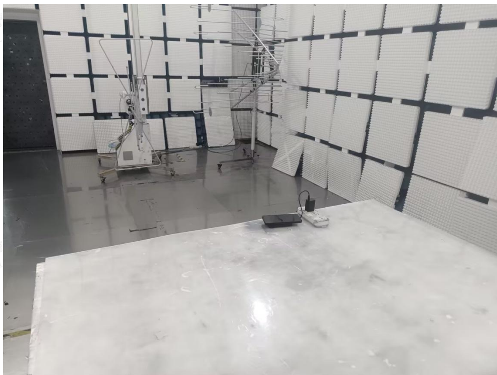
Radiated Emission below 1GHz-AC adapter charge mode
