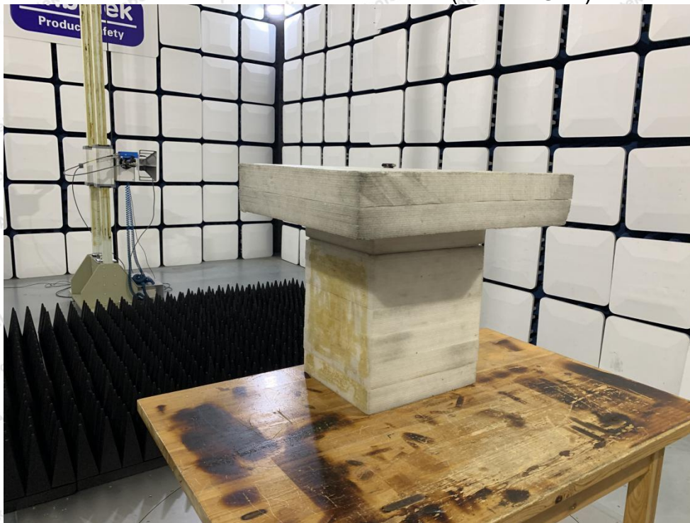
Photo of Radiation Emission Test (above 1GHz)
