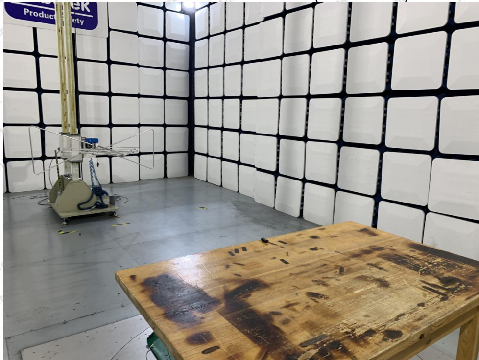
Photo of Radiation Emission Test (below 1GHz)
