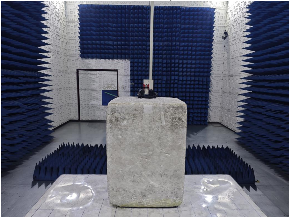
Radiated Emission Test Setup 1GHz-18GHz
