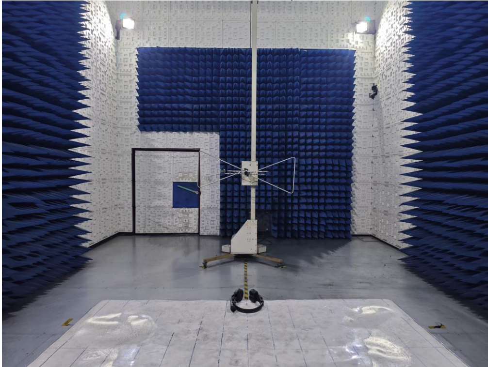
Radiated Emission Test Setup 1GHz-18GHz
