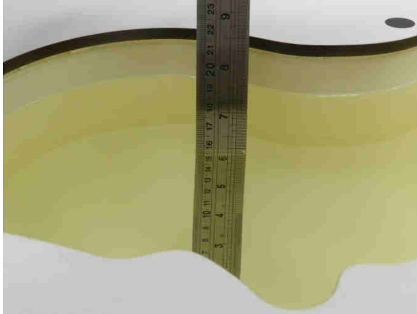
Fig 10.1 Photo of Liquid Height for Head SAR
