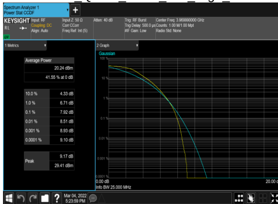
N77(20M)_DFT-s-OFDM QPSK Outer Full High CH
