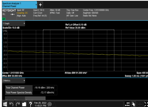
B66_N25(20M)_DFT-s- OFDM_QPSK_Edge_1RB_Right_High_CH_chp _PASS
