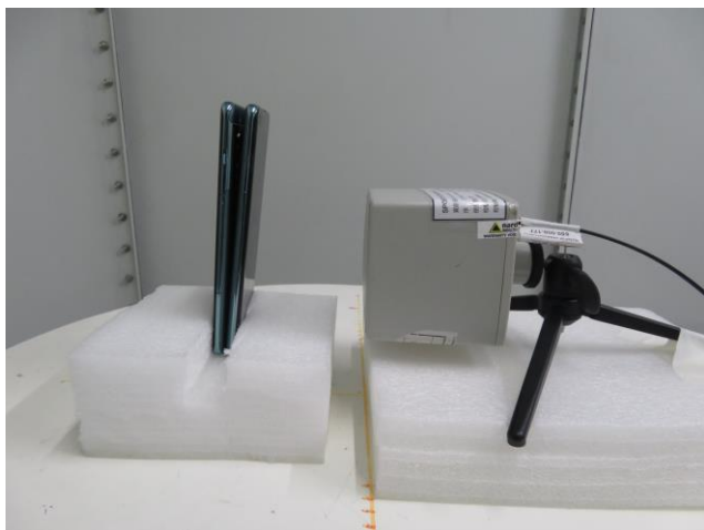
Position A, test separation 10cm
