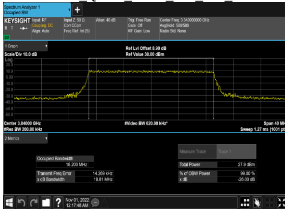
N77(20M)_CP- OFDM QPSK Outer Full Mid CH
