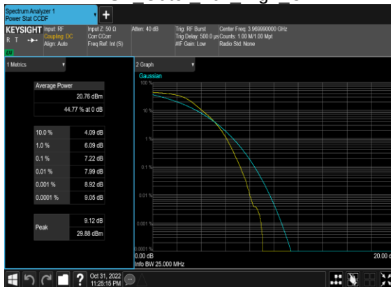
N77(20M)_DFT-s-OFDM_PI_2-BPSK Outer Full High CH
