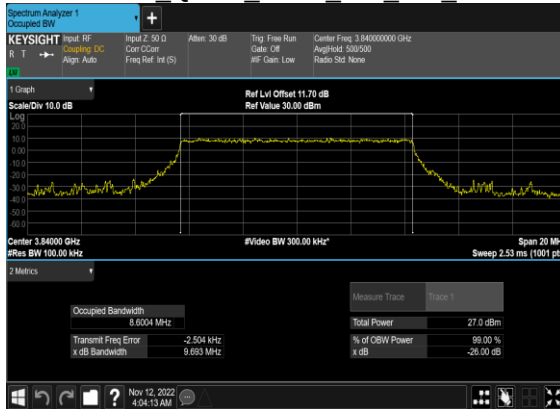
N77(10M)_CP- OFDM QPSK Outer Full Mid CH
