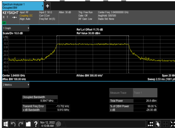
N77(10M)_CP-OFDM_64 QAM Outer Full Mid CH
