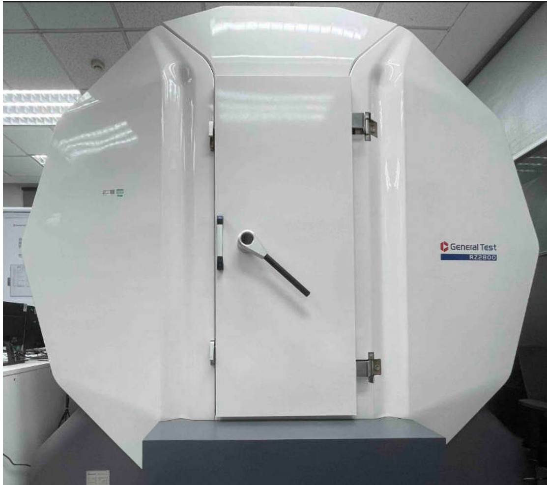
Fig. 5. The fully anechoic chamber
