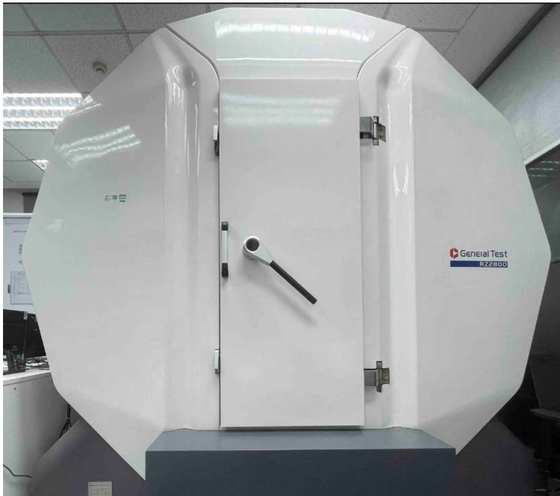
Fig. 5. The fully anechoic chamber
