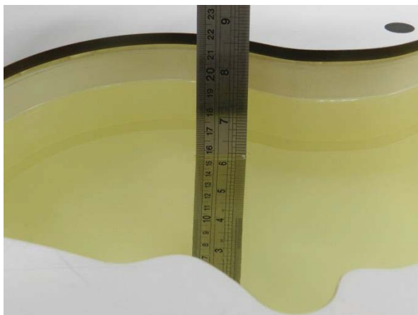
Fig 10.1 Photo of Liquid Height for Head SAR
