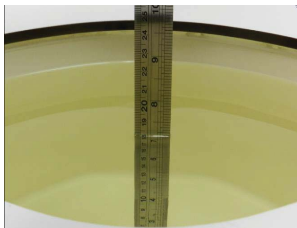
Fig 10.2 Photo of Liquid Height for Body SAR
