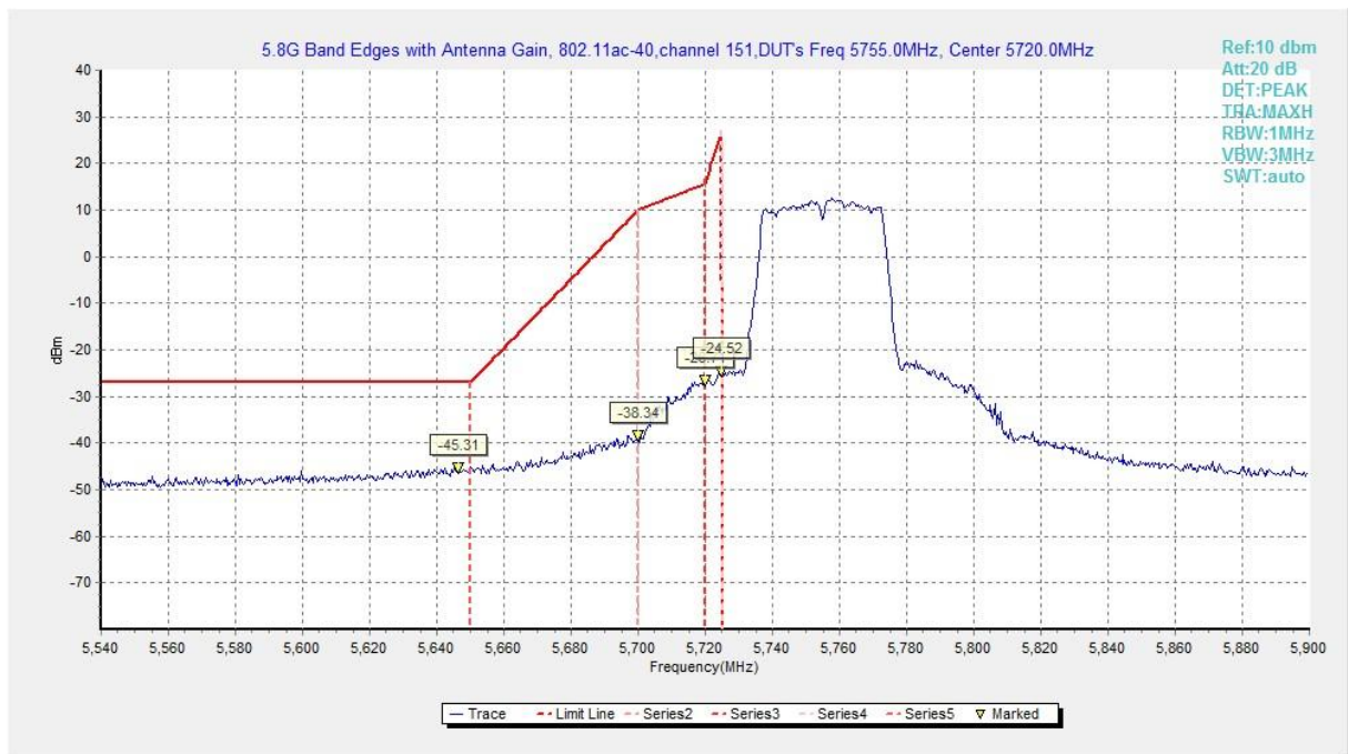
Fig. 79 Band Edges (802.11ac-HT40, 5755MHz)
