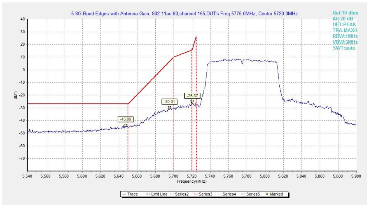
Fig. 81 Band Edges (802.11ac-HT80, 5775MHz)
