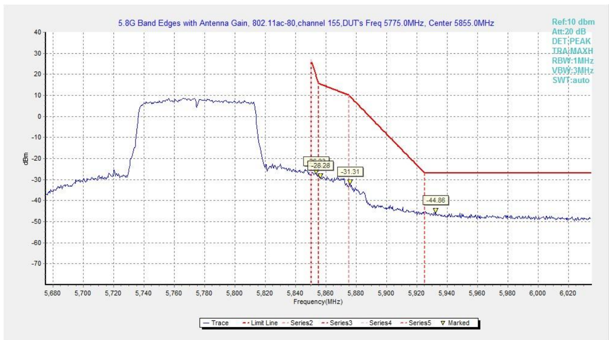
Fig. 82 Band Edges (802.11ac-HT80, 5775MHz)
