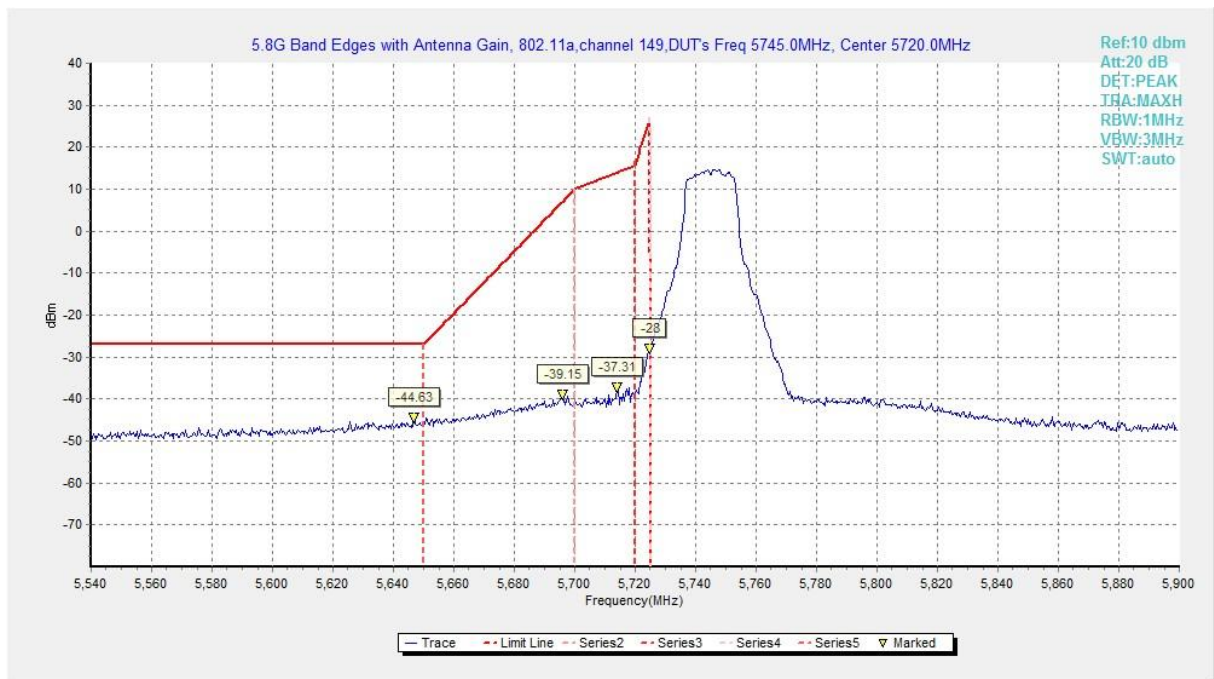
Fig. 71 Band Edges (802.11a, 5745MHz)
