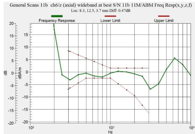
Figure C.26 Frequency Response of WiFi-2.4G - OTT VoIP
