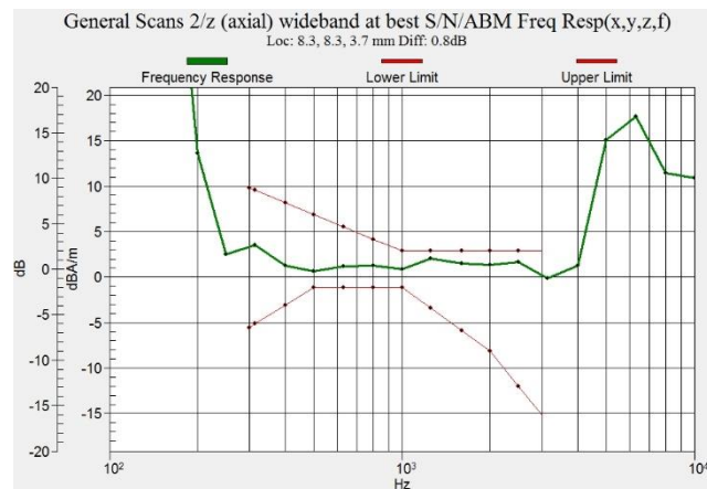
Figure C.8 Frequency Response of CDMA BC10
