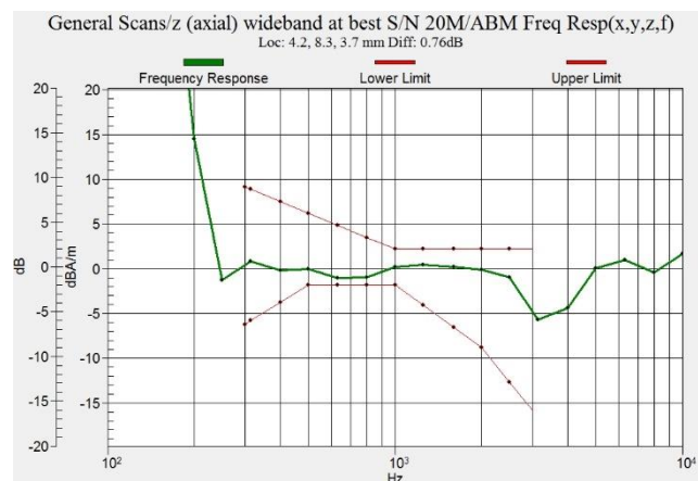
Figure C.15 Frequency Response of LTE B66
