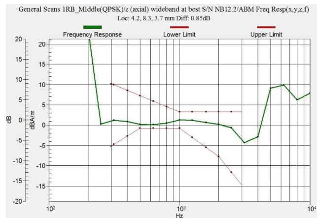
Figure C.17 Frequency Response of LTE B41 Power Class 2
