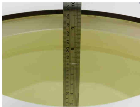
Fig 10.2 Photo of Liquid Height for Body SAR
