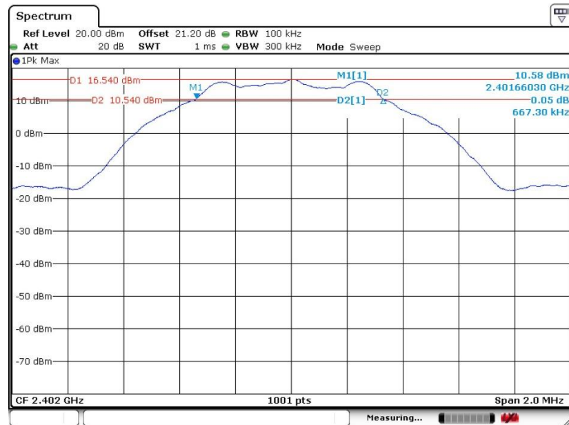
6 dB Bandwidth Plot on Channel 00
