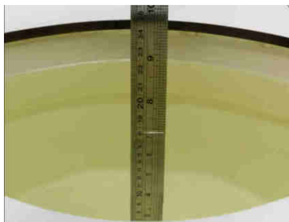
Fig 10.2 Photo of Liquid Height for Body SAR
