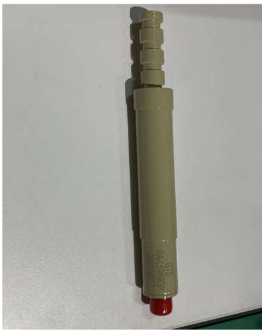
Fig 3 dipole model RA-L5969DP frequency 5900~6900 MHz
