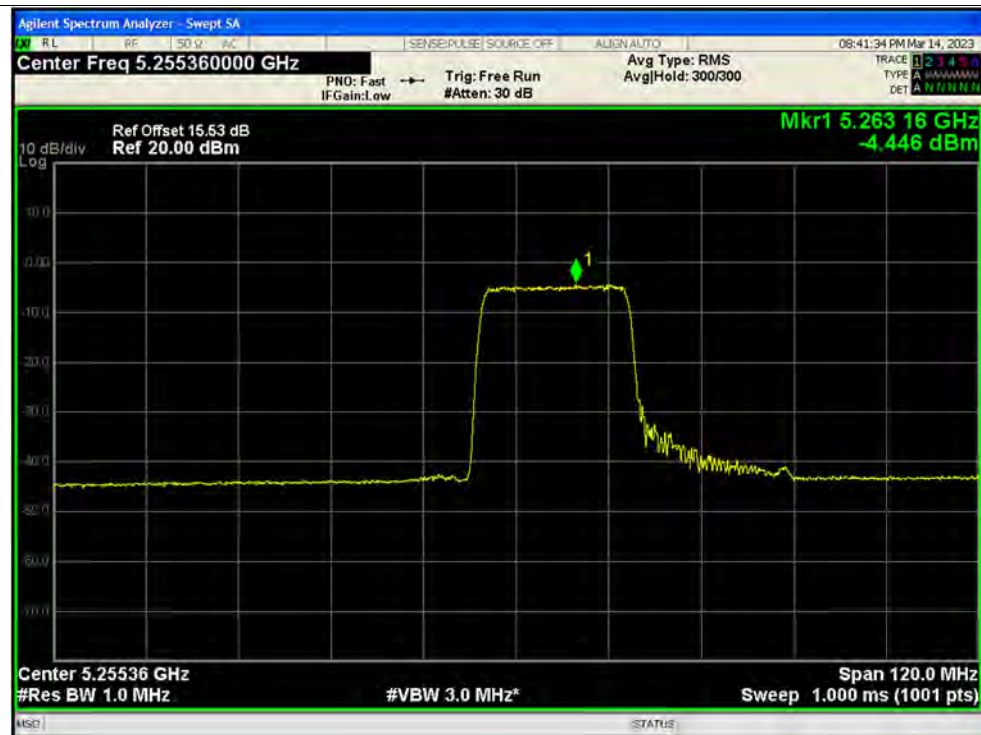
PSD NVNT ax80 242@61 5290MHz Ant3
