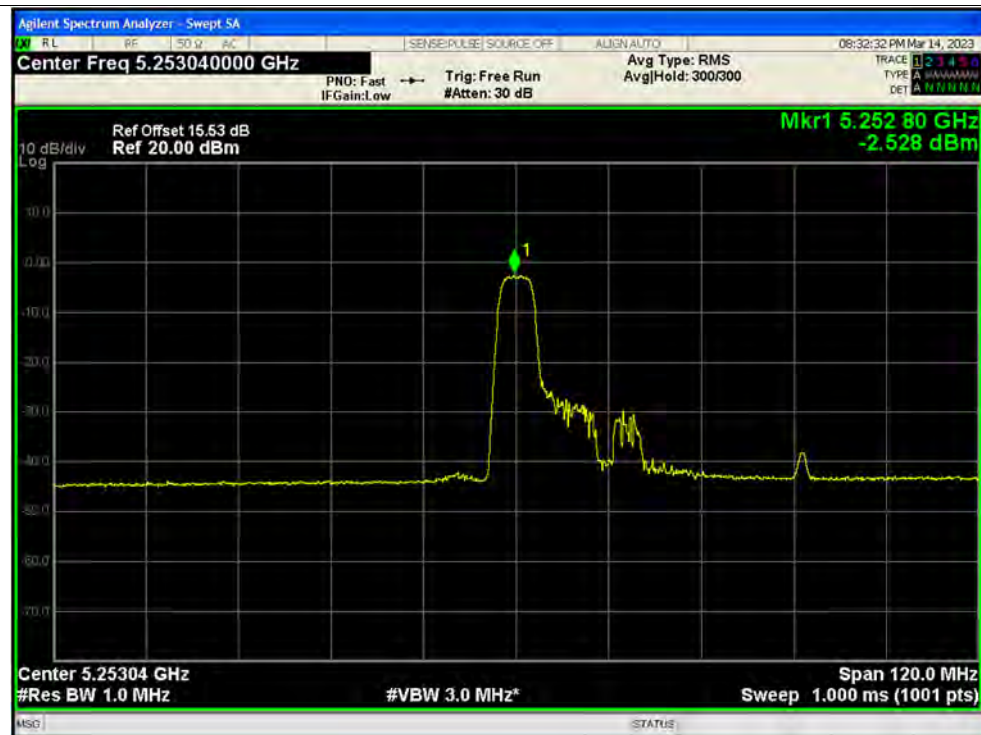
PSD NVNT ax80 52@37 5290MHz Ant3
