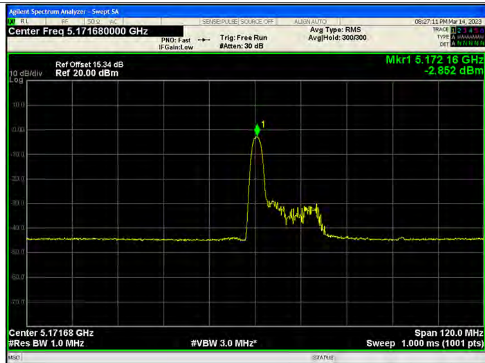
PSD NVNT ax80 26@0 5210MHz Ant3
