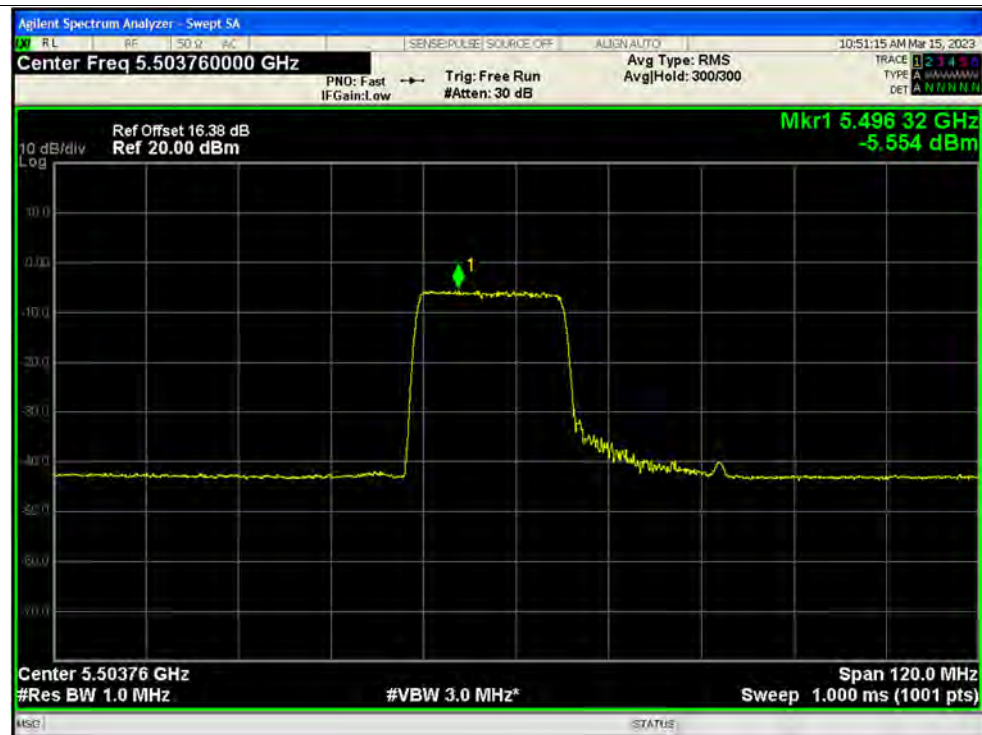
PSD NVNT ax80 242@61 5530MHz Ant3
