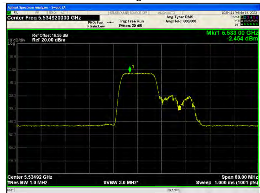
PSD NVNT ax40 106@53 5550MHz Ant3
