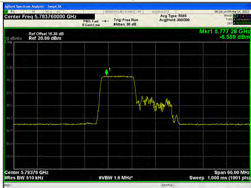
PSD NVNT ax40 106@53 5795MHz Ant3
