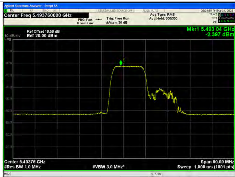
PSD NVNT ax40 106@53 5510MHz Ant3
