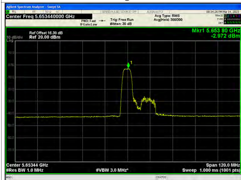
PSD NVNT ax80 52@37 5690MHz Ant3
