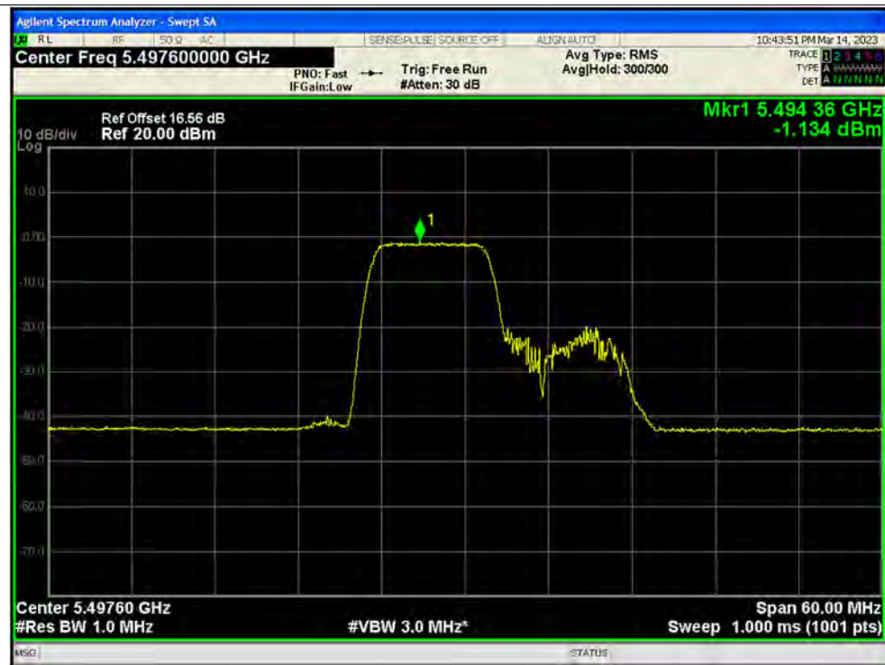
PSD NVNT ax40 106@53 5510MHz Ant3
