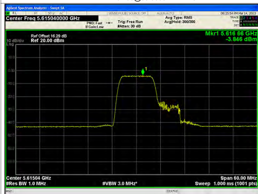
PSD NVNT ax40 106@53 5630MHz Ant3
