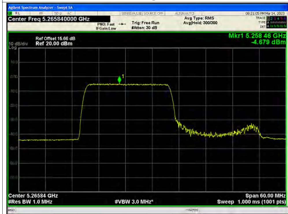
PSD NVNT ax40 242@61 5270MHz Ant3
