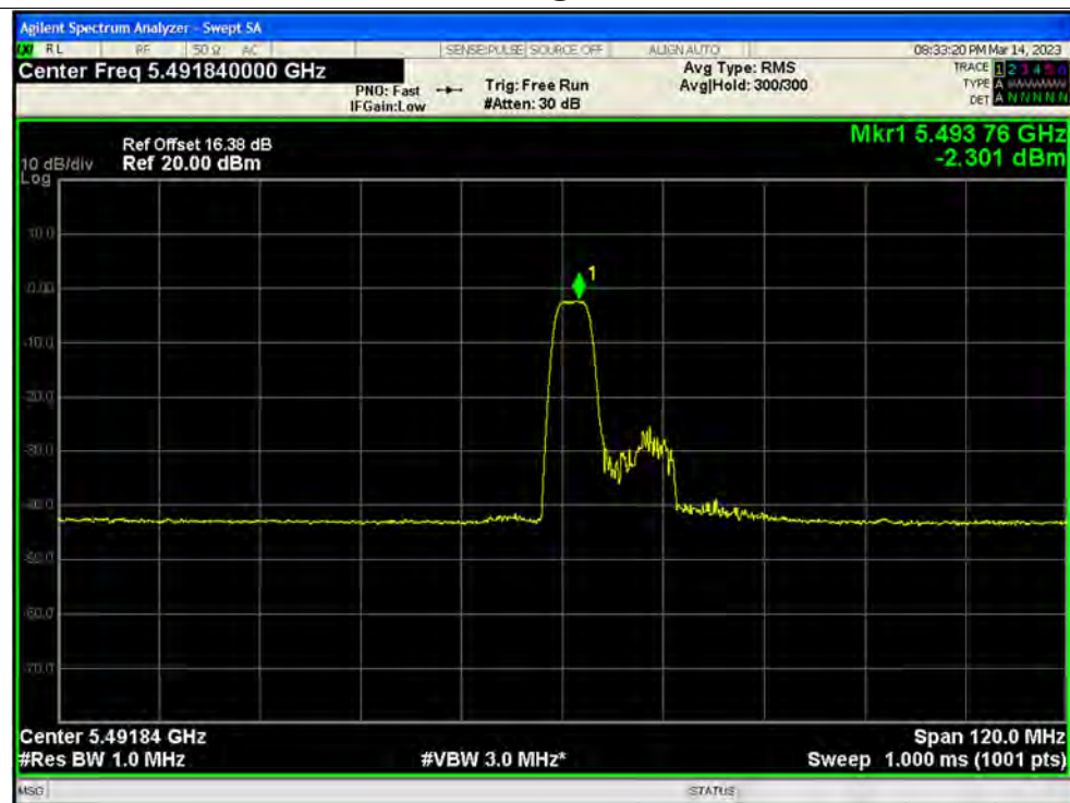
PSD NVNT ax80 52@37 5530MHz Ant3
