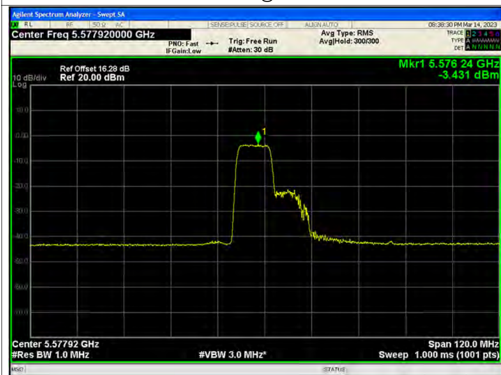
PSD NVNT ax80 106@53 5610MHz Ant3
