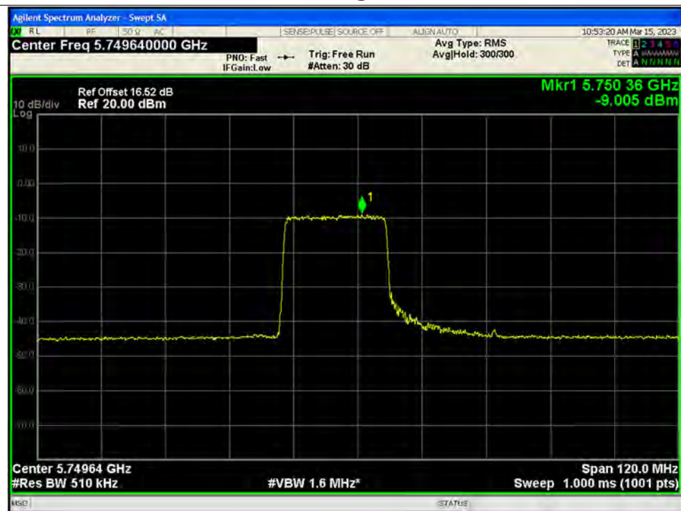
PSD NVNT ax80 242@61 5775MHz Ant3
