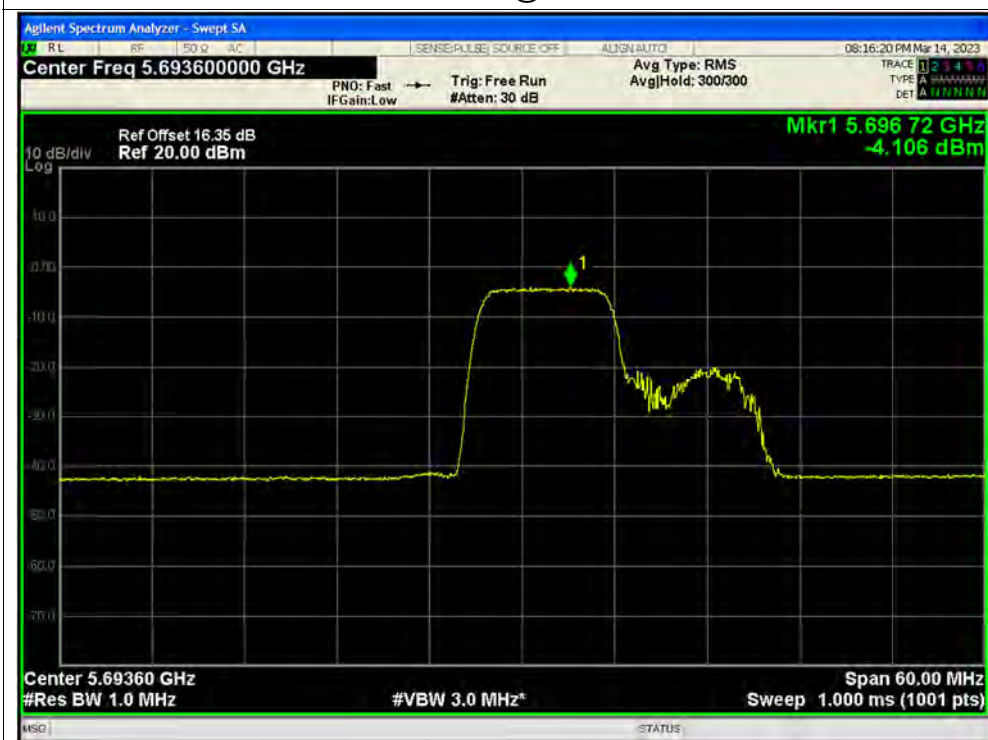
PSD NVNT ax40 106@53 5710MHz Ant3
