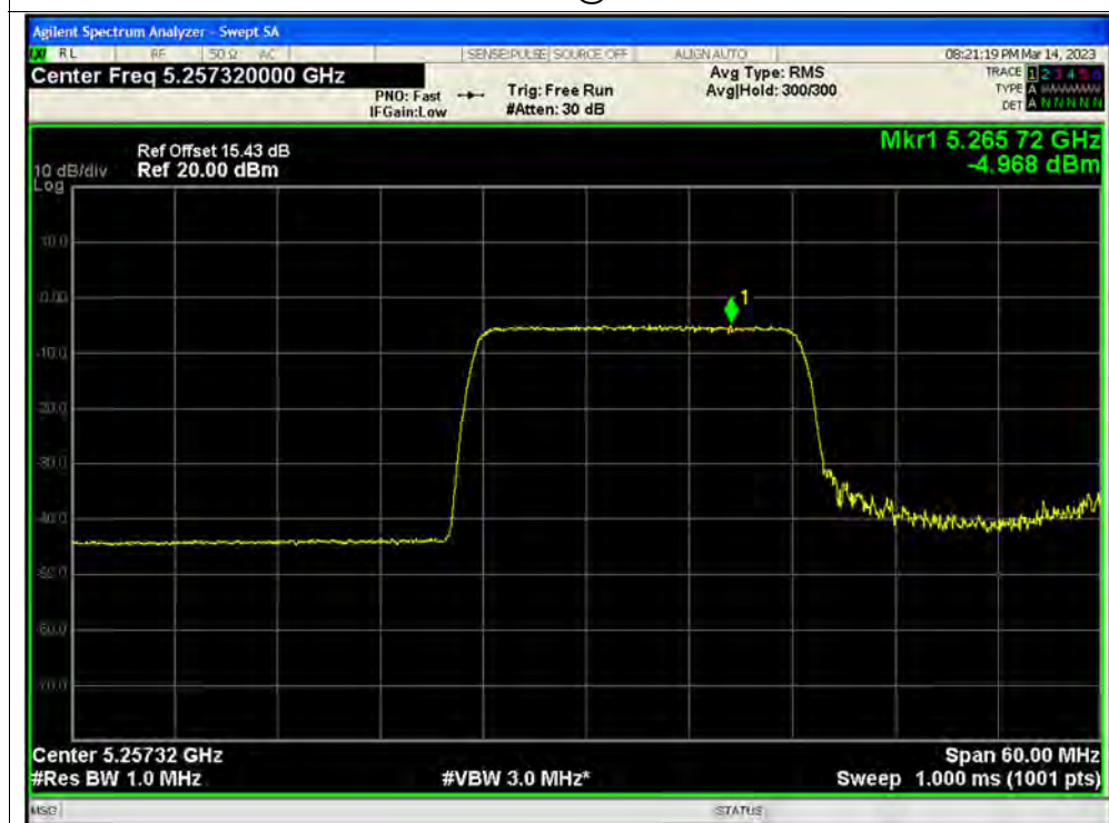
PSD NVNT ax40 242@61 5270MHz Ant3
