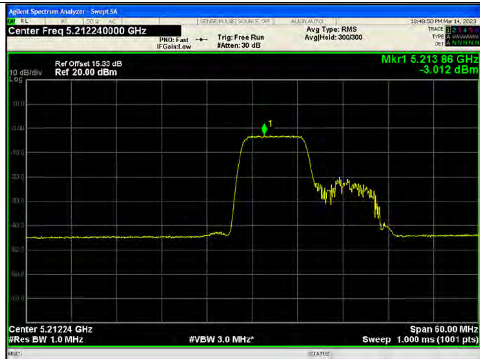
PSD NVNT ax40 106@53 5230MHz Ant3
