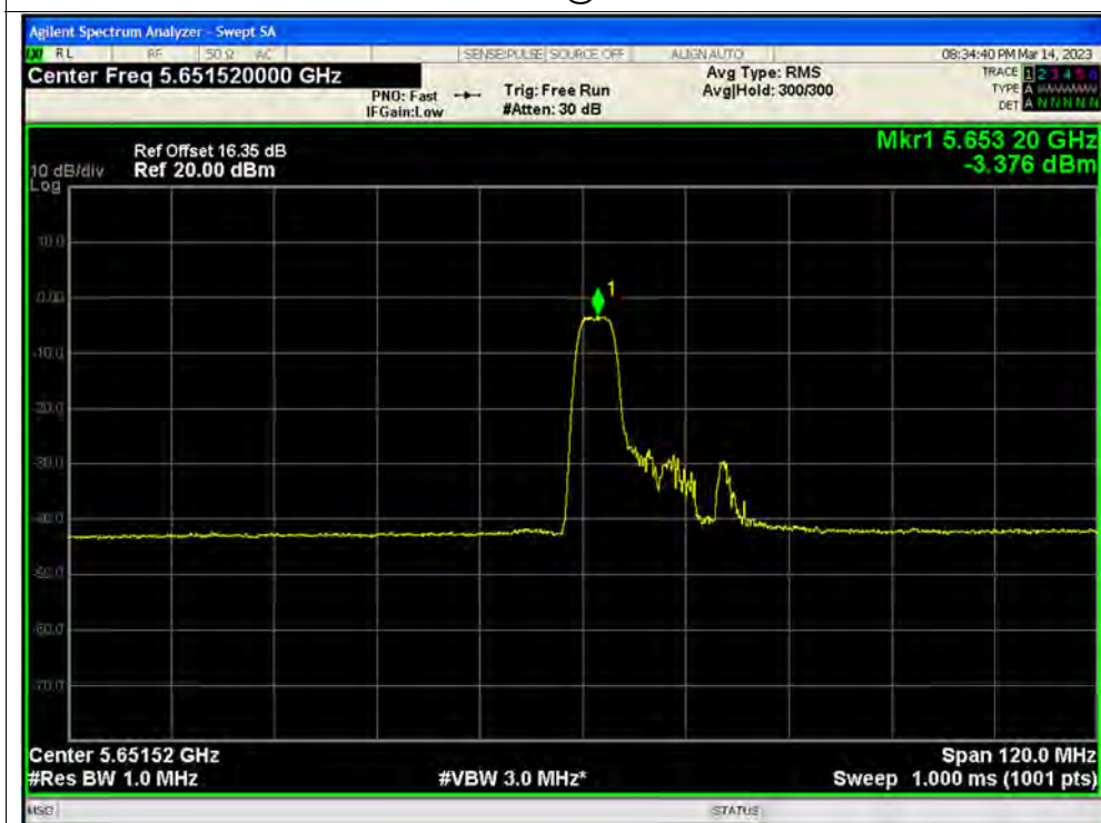
PSD NVNT ax80 52@37 5690MHz Ant3
