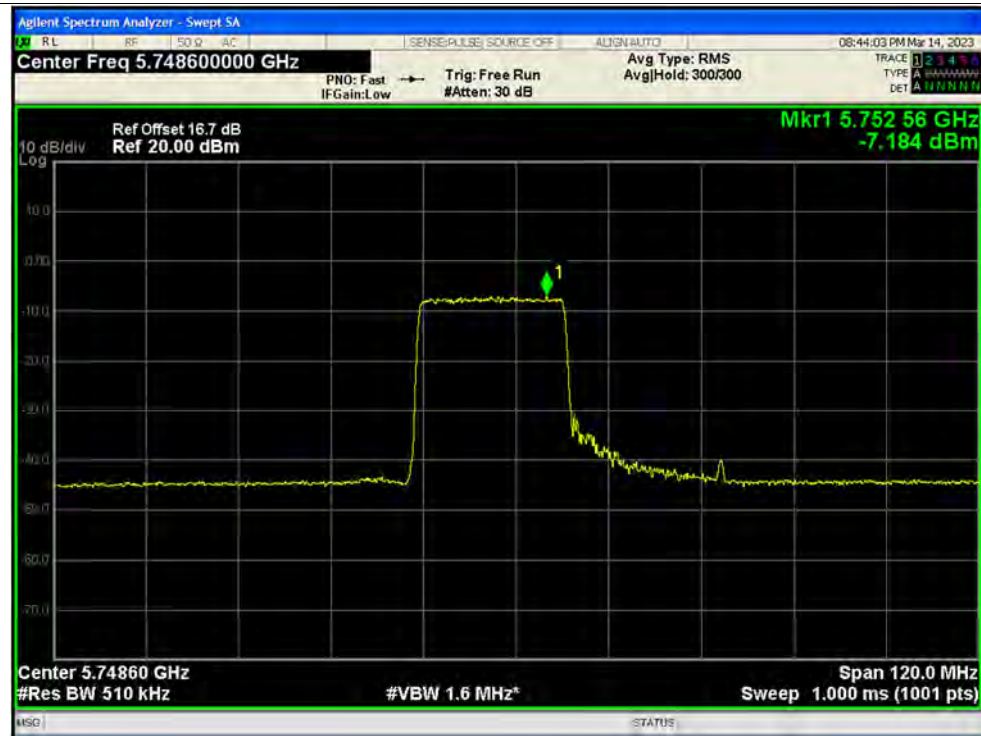
PSD NVNT ax80 242@61 5775MHz Ant3
