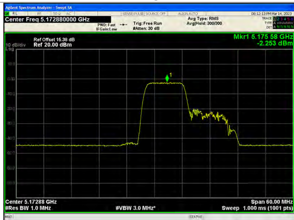
PSD NVNT ax40 106@53 5190MHz Ant3
