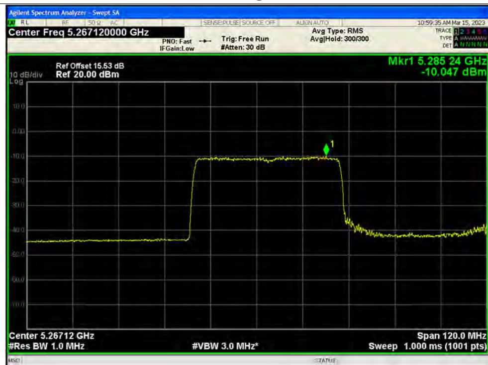
PSD NVNT ax80 242@65 5290MHz Ant3
