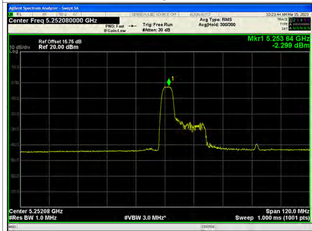
PSD NVNT ax80 52@37 5290MHz Ant3
