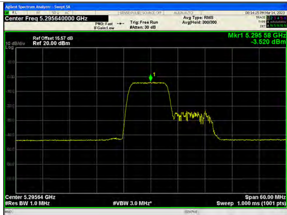
PSD NVNT ax40 106@53 5310MHz Ant3
