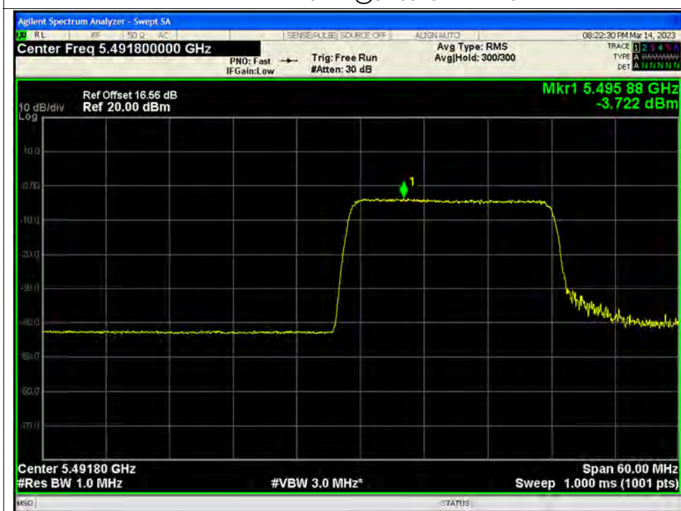
PSD NVNT ax40 242@61 5510MHz Ant3
