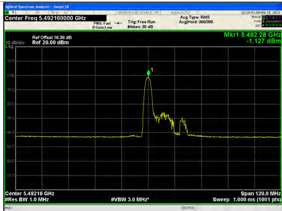
PSD NVNT ax80 26@0 5530MHz Ant3
