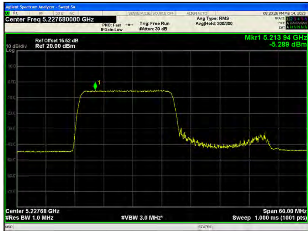
PSD NVNT ax40 242@61 5230MHz Ant3
