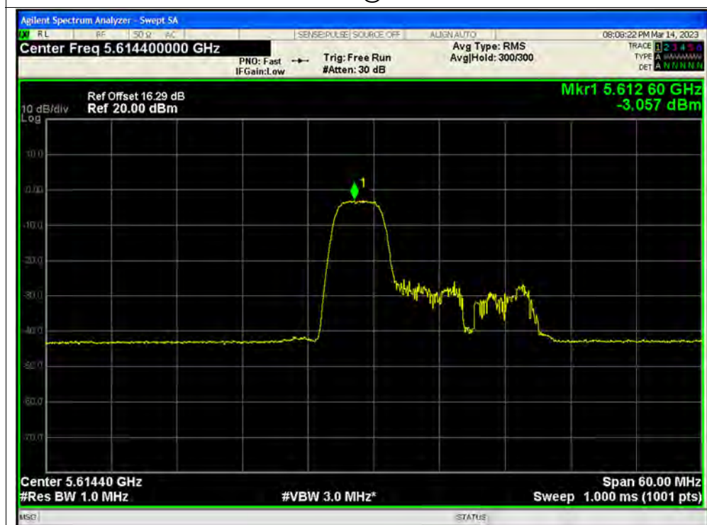
PSD NVNT ax40 52@37 5630MHz Ant3
