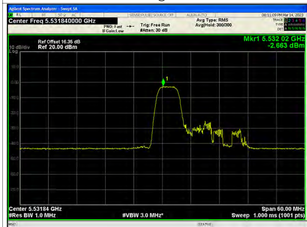
PSD NVNT ax40 52@37 5550MHz Ant3
