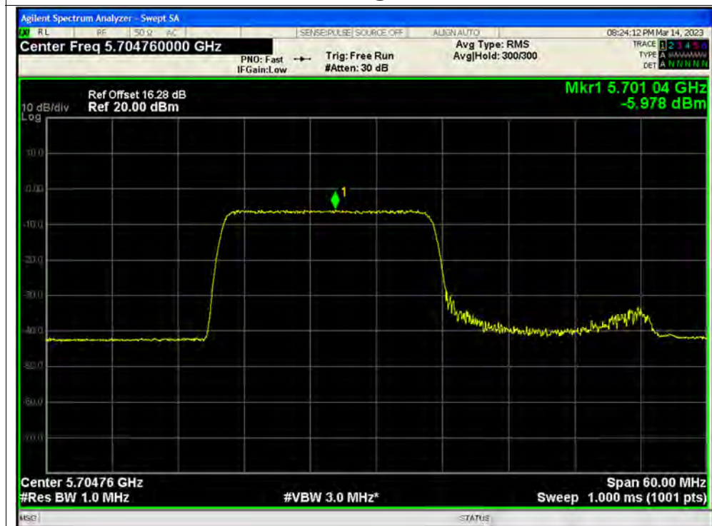
PSD NVNT ax40 242@61 5710MHz Ant3
