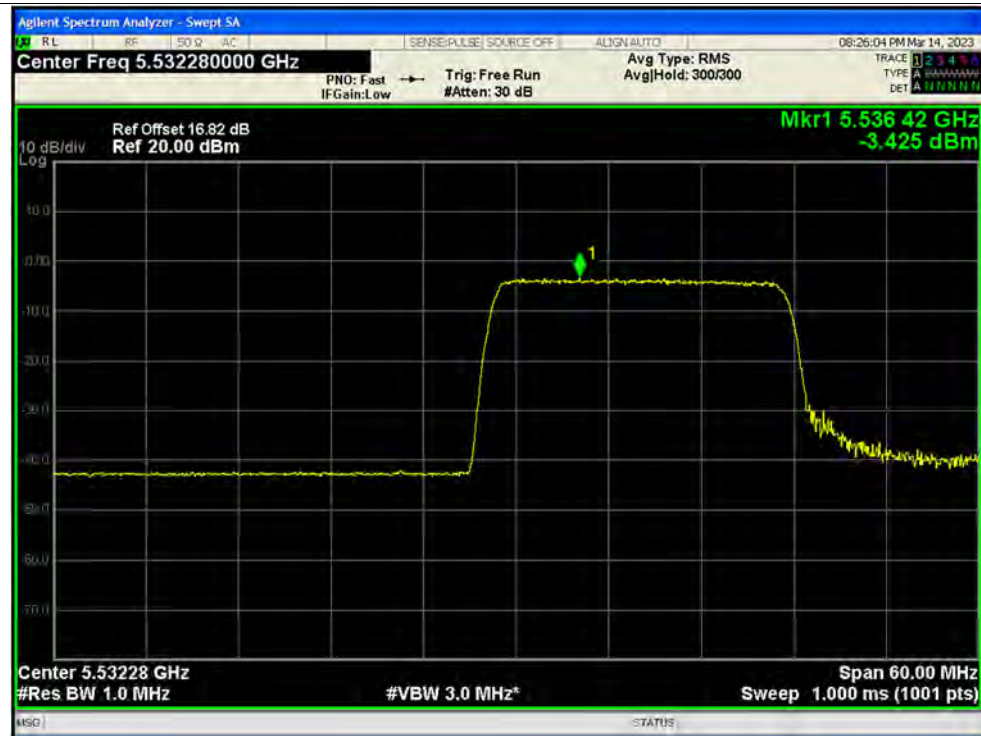
PSD NVNT ax40 242@61 5550MHz Ant3
