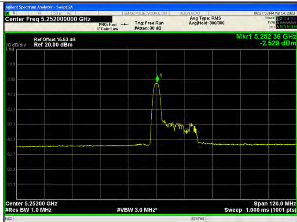
PSD NVNT ax80 26@0 5290MHz Ant3
