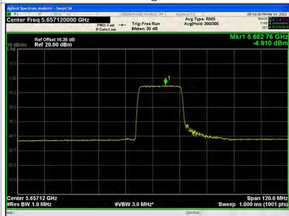
PSD NVNT ax80 242@61 5690MHz Ant3
