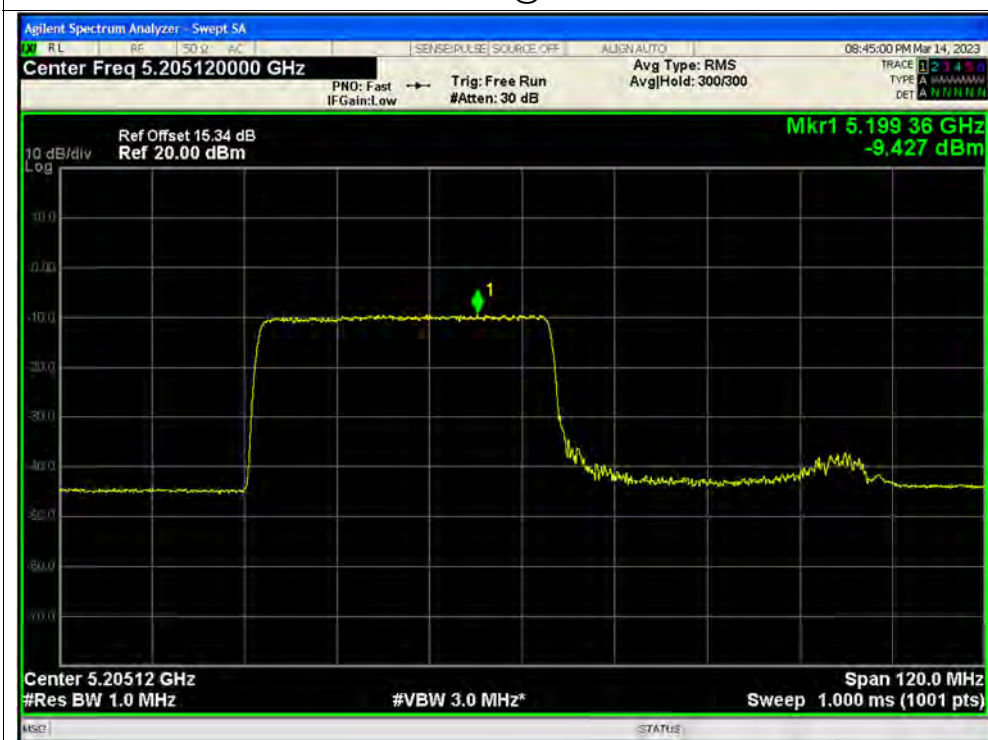
PSD NVNT ax80 242@65 5210MHz Ant3
