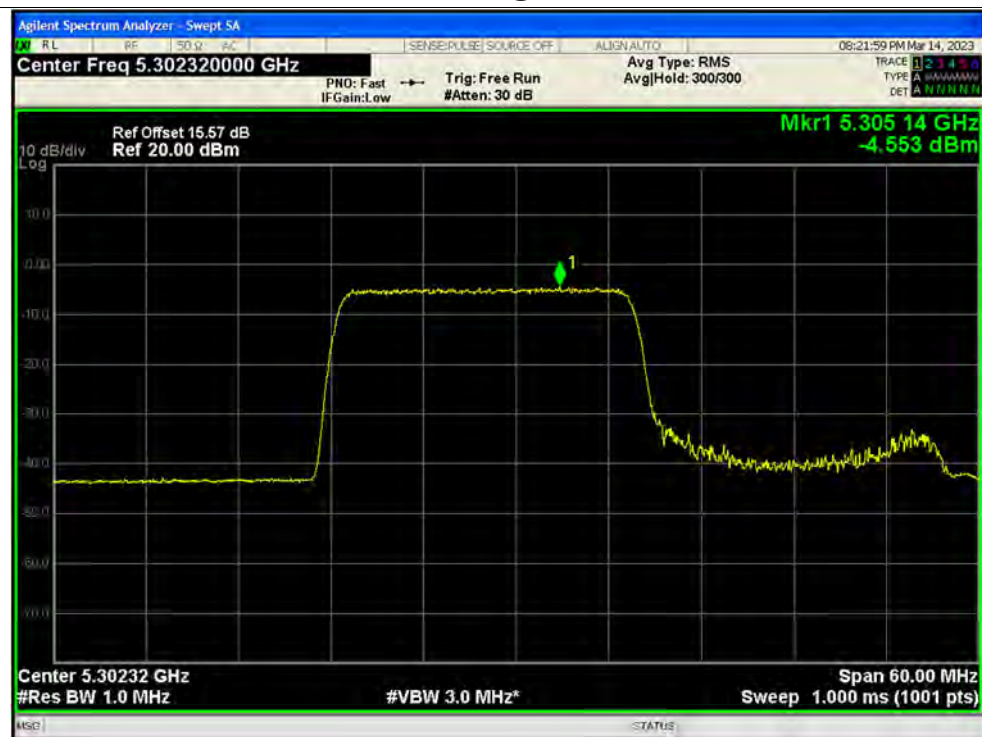
PSD NVNT ax40 242@61 5310MHz Ant3
