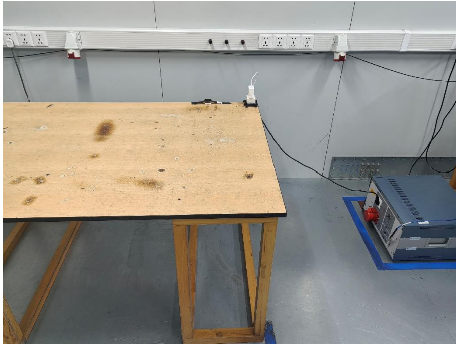
AC Conducted Emission Test Setup -Front
