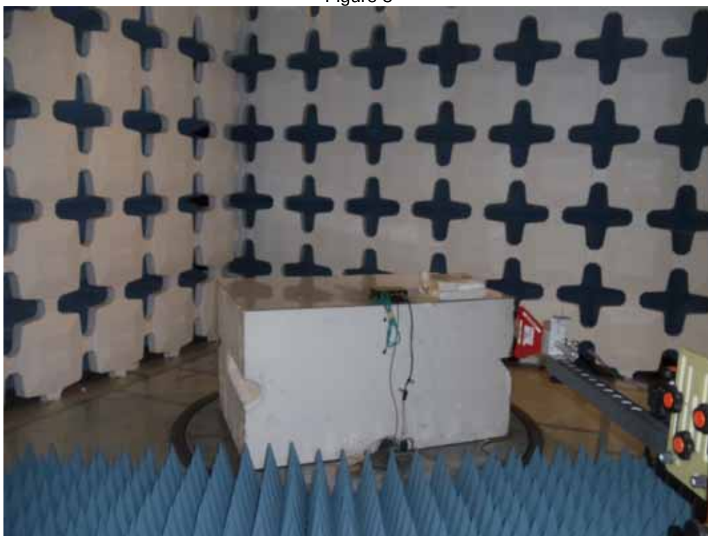
Test Setup for Radiated Emissions, Above 1GHz – Horizontal Polarization at 1Meter
