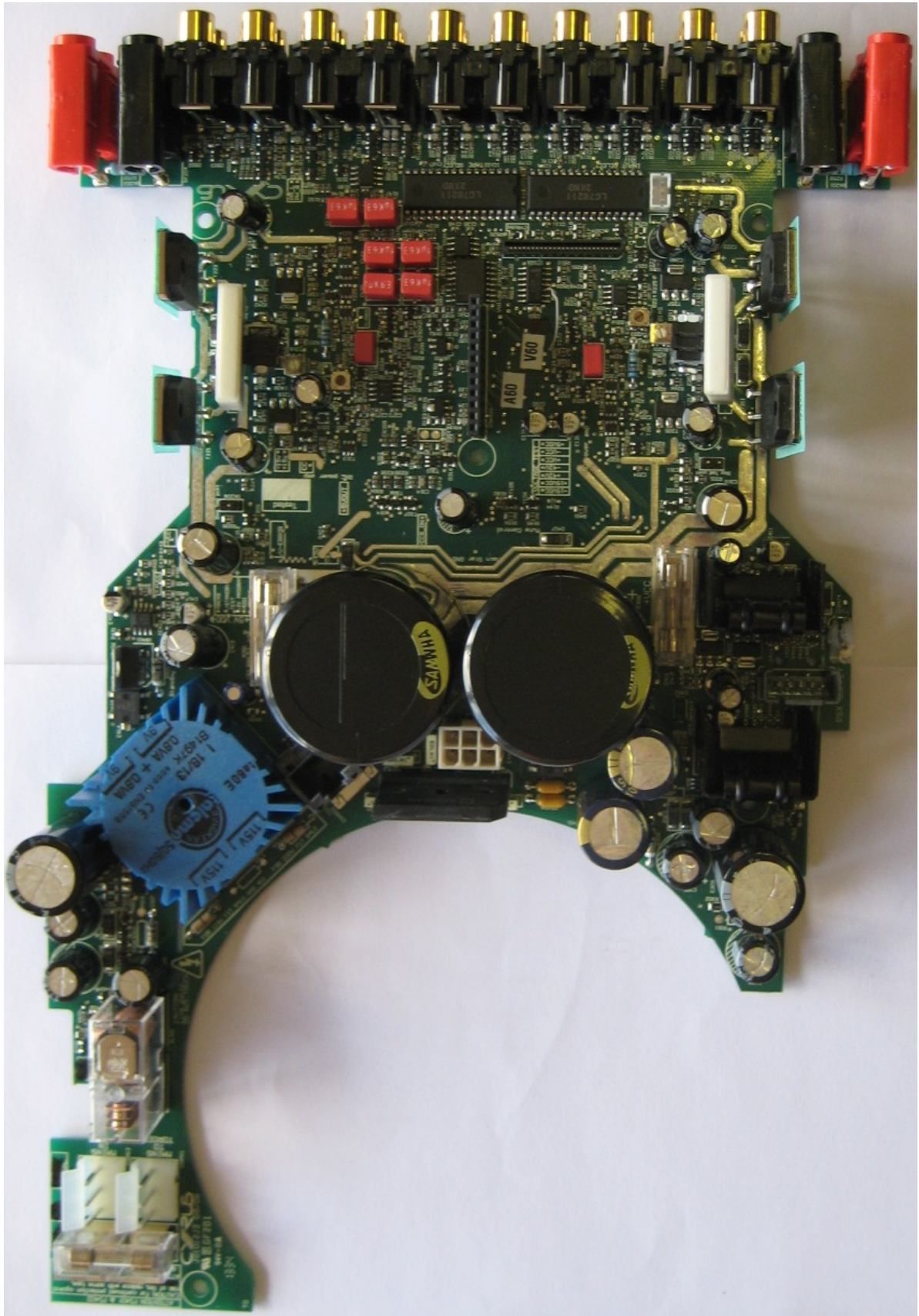
5. Main PCB Component Side: Cyrus 6 DAC and Cyrus 8 DAC
