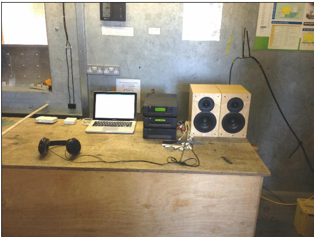
Photograph 4 Conducted Emissions - 8dac - USB Source
