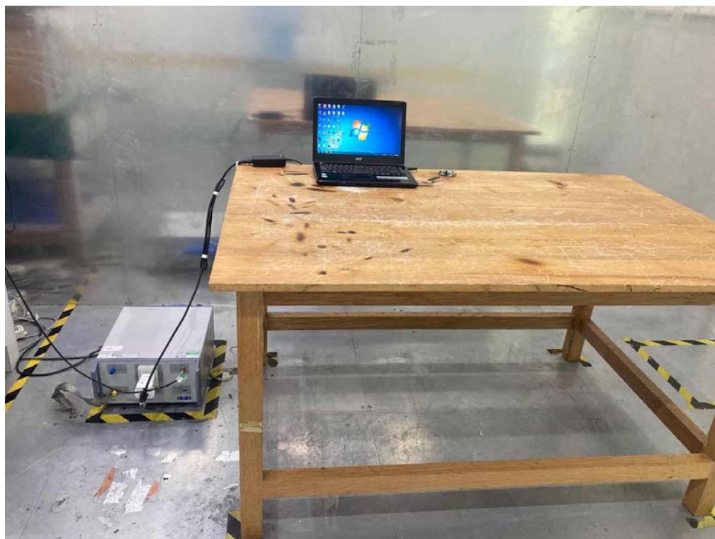
Conducted Emission Test Photo
