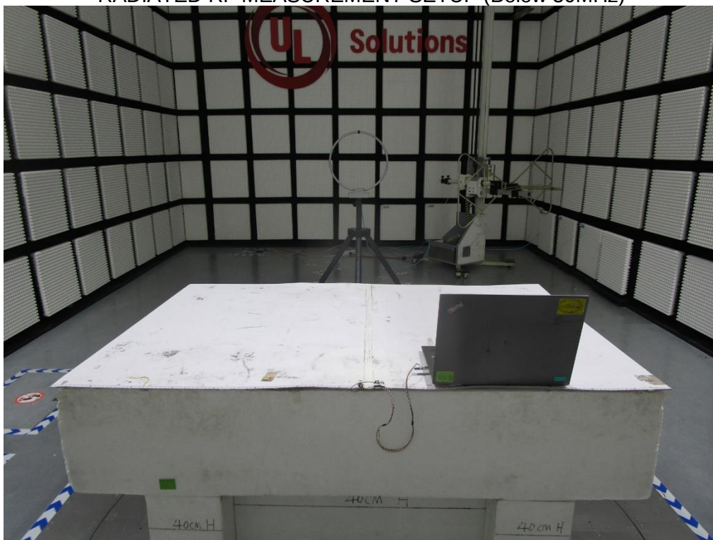
RADIATED RF MEASUREMENT SETUP (Below 30MHz)
