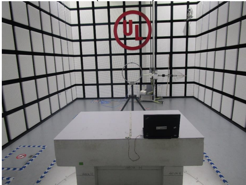
RADIATED RF MEASUREMENT SETUP (Below 30 MHz) (PCB Antenna)
