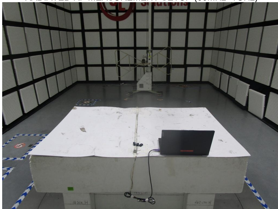
RADIATED RF MEASUREMENT SETUP (Below 30MHz)
