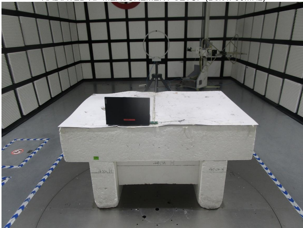
RADIATED RF MEASUREMENT SETUP (Below 30MHz)
