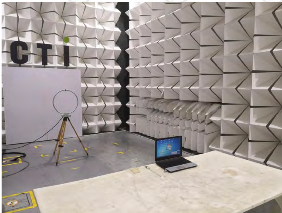
Radiated spurious emission Test Setup-1(Below 30MHz)
