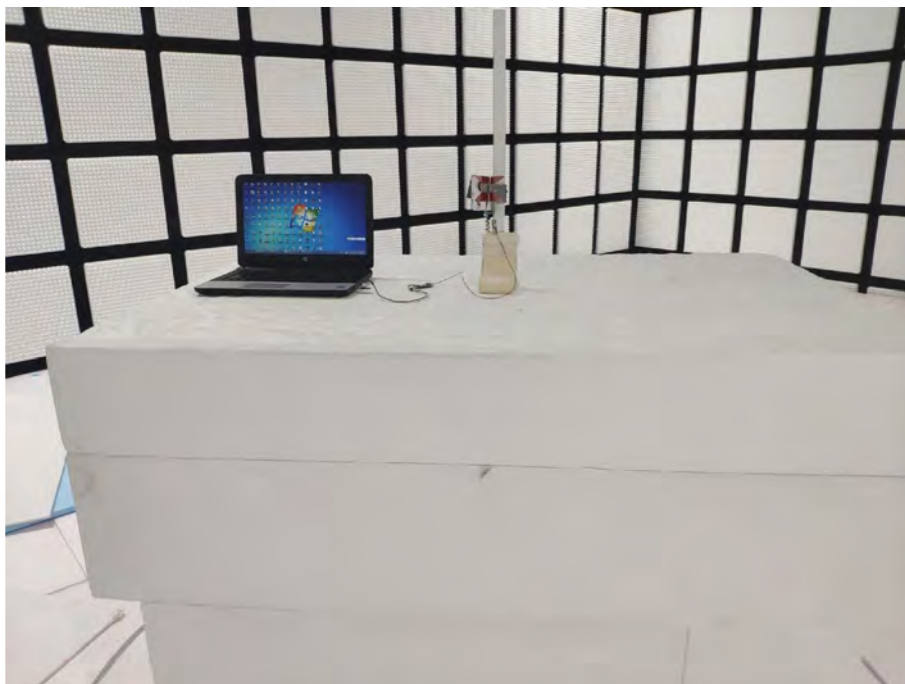
Radiated spurious emission Test Setup-3(Above 1GHz)
