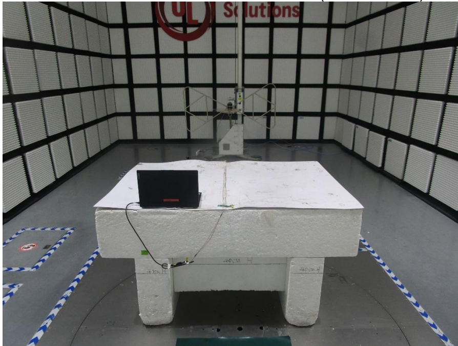
RADIATED RF MEASUREMENT SETUP (Below 30MHz)
