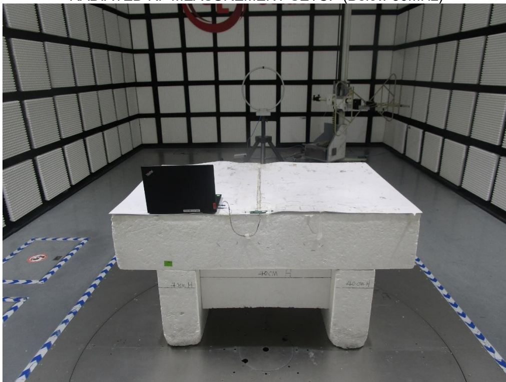
RADIATED RF MEASUREMENT SETUP (Below 30MHz)
