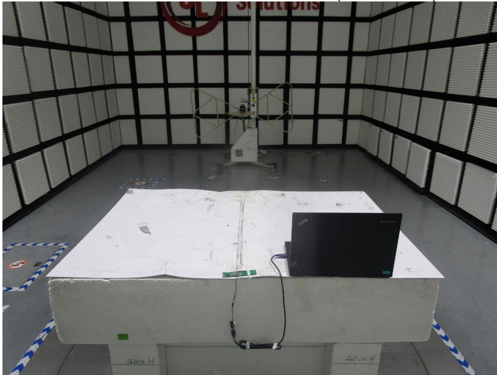
RADIATED RF MEASUREMENT SETUP (Below 30MHz)
