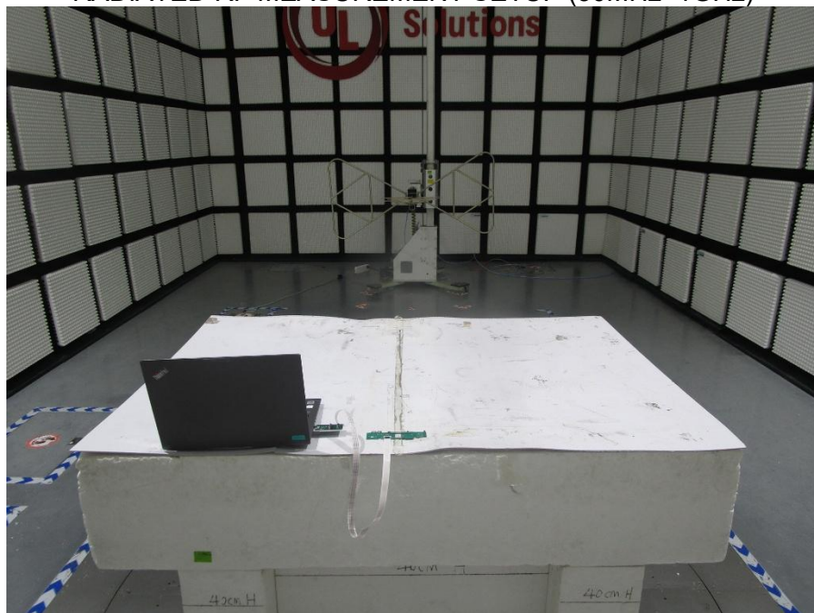
RADIATED RF MEASUREMENT SETUP (Below 30MHz)
