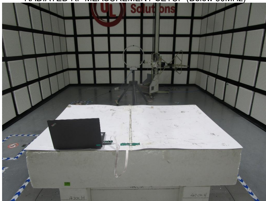
RADIATED RF MEASUREMENT SETUP (Below 30MHz)
