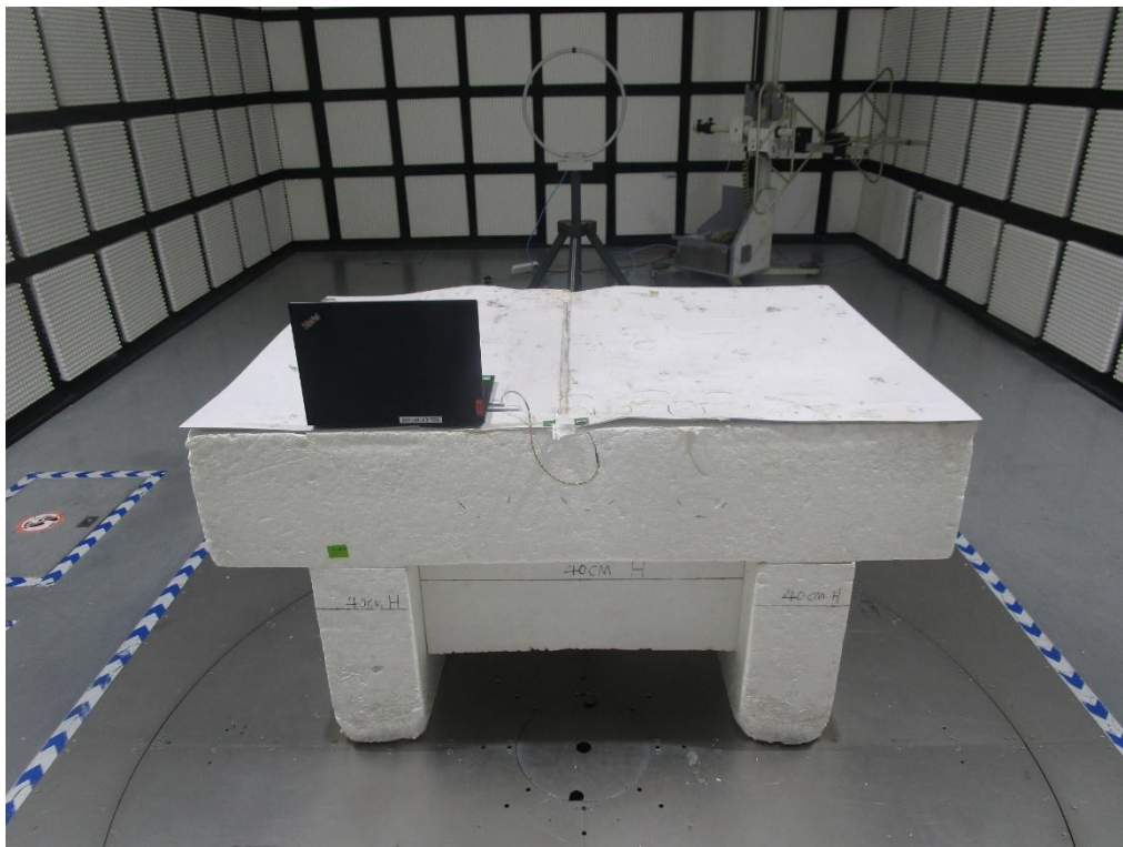
RADIATED RF MEASUREMENT SETUP (Below 30MHz)
