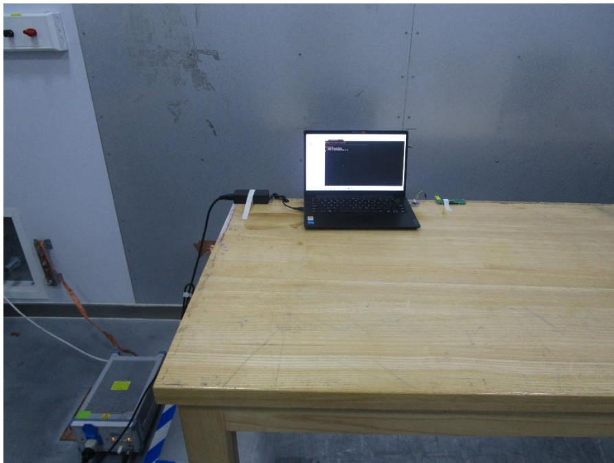
POWERLINE CONDUCTED EMISSIONS MEASUREMENT SETUP
