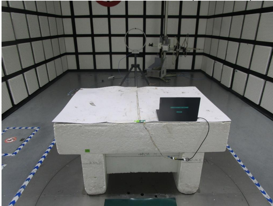
POWERLINE CONDUCTED EMISSIONS MEASUREMENT SETUP
