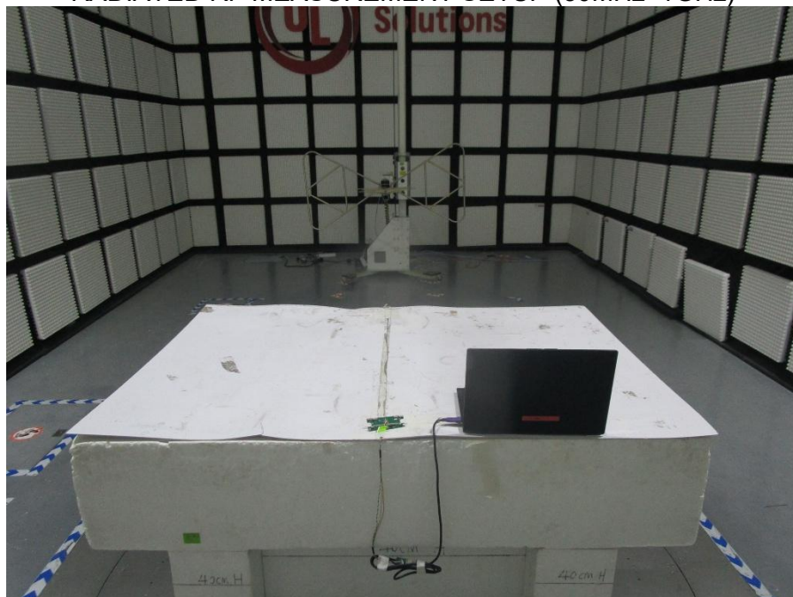
RADIATED RF MEASUREMENT SETUP (Below 30MHz)
